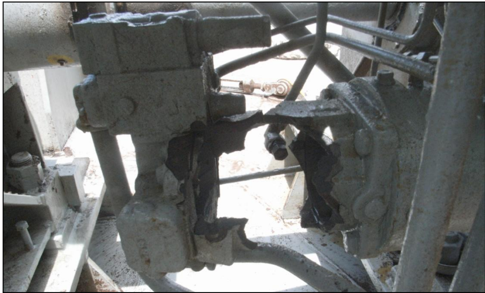
Figure 8: Shattered casing of windlass hydraulic motor
