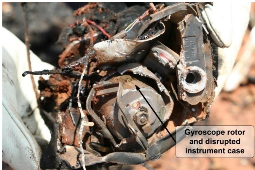
Figure 3: Directional indicator with gyroscope rotor and disrupted instrument case
