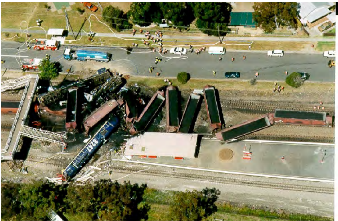
Figures 4 and 5 showing wreckage distribution. Overhead bridge is located at eastern end of platform.
