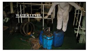
At 1945, engineers removed the after peak WBTK manhole cover and began to pump the water from the engine room into the after peak tank using a submersible pump and hoses.
