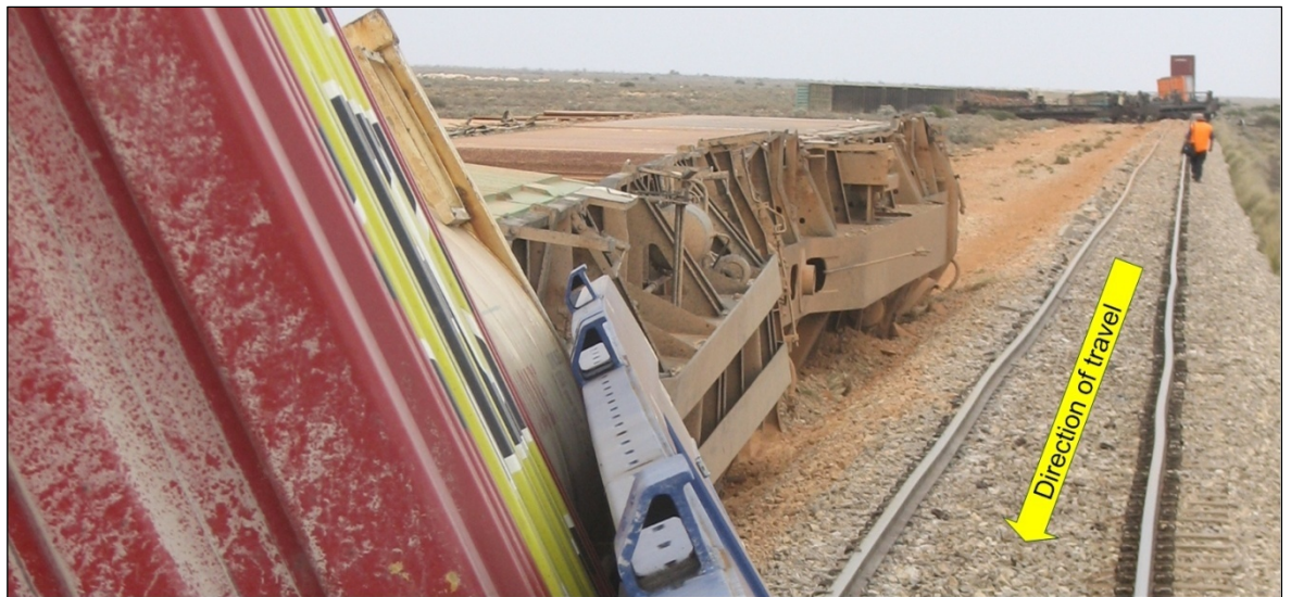
Figure 1: Derailment site showing separated front and rear portions of train 2PM6.
