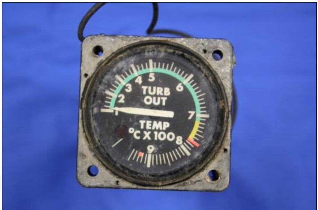
Figure 2: Turbine outlet temperature gauge (TOT)
