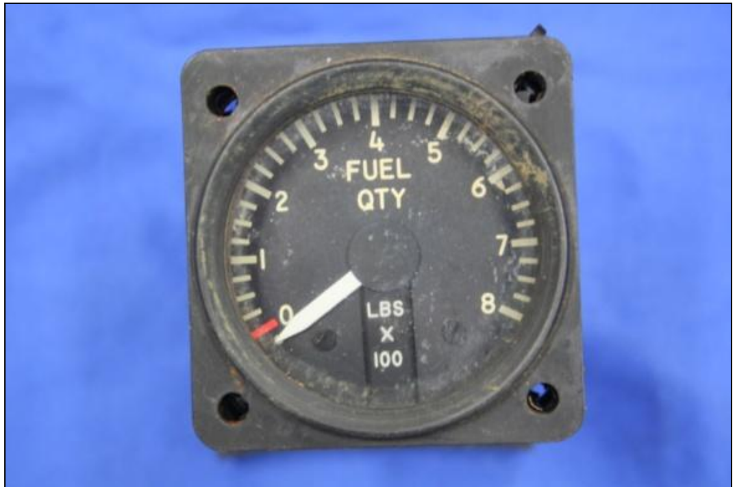
Figure 1: Fuel quantity gauge
