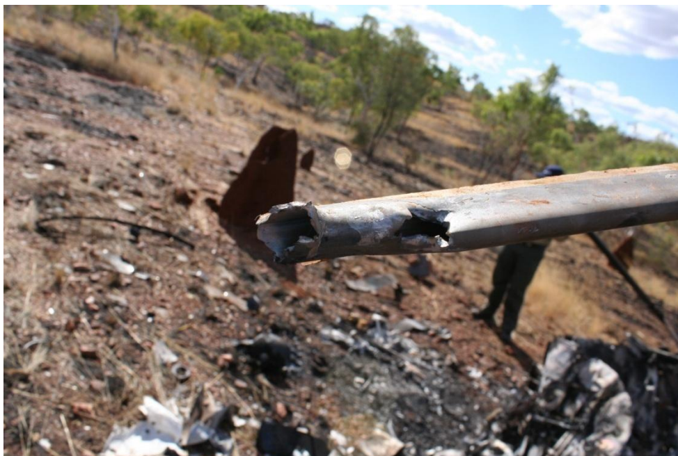
Figure 5: Missing blade tip and notched leading edge
