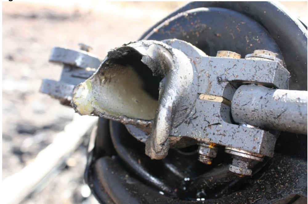
Figure 7: Failed rotor mast
