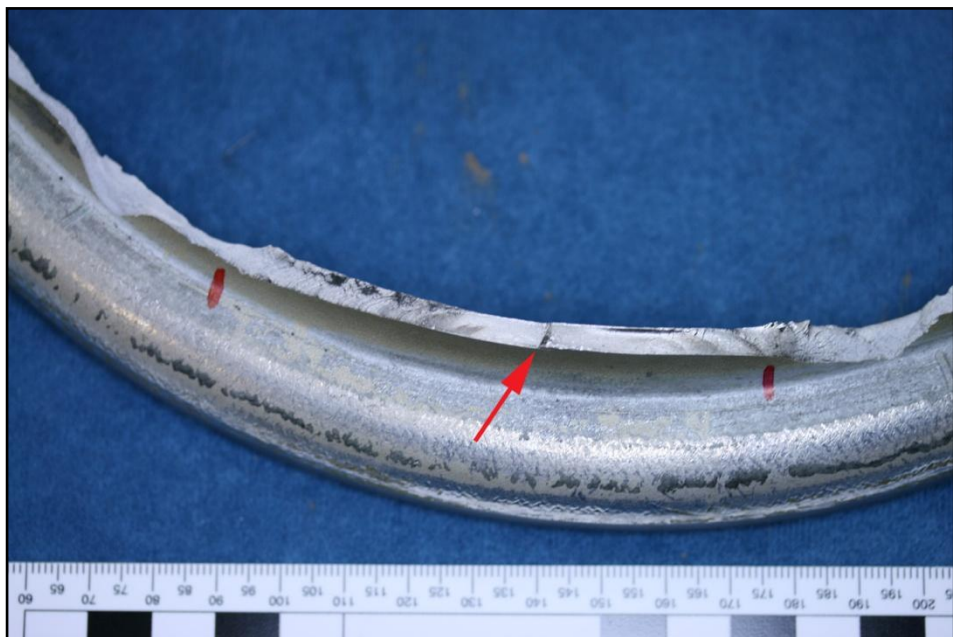
Figure 3: Magnified view of fracture face showing the crack progression (beach-marks) extending from the bead seat radius origin area (arrowed)
