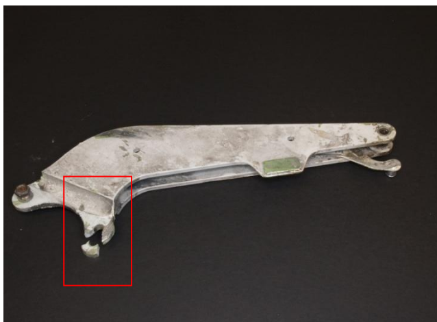
Figure 4: Inboard auxiliary track showing failed bolt hole (highlighted)
