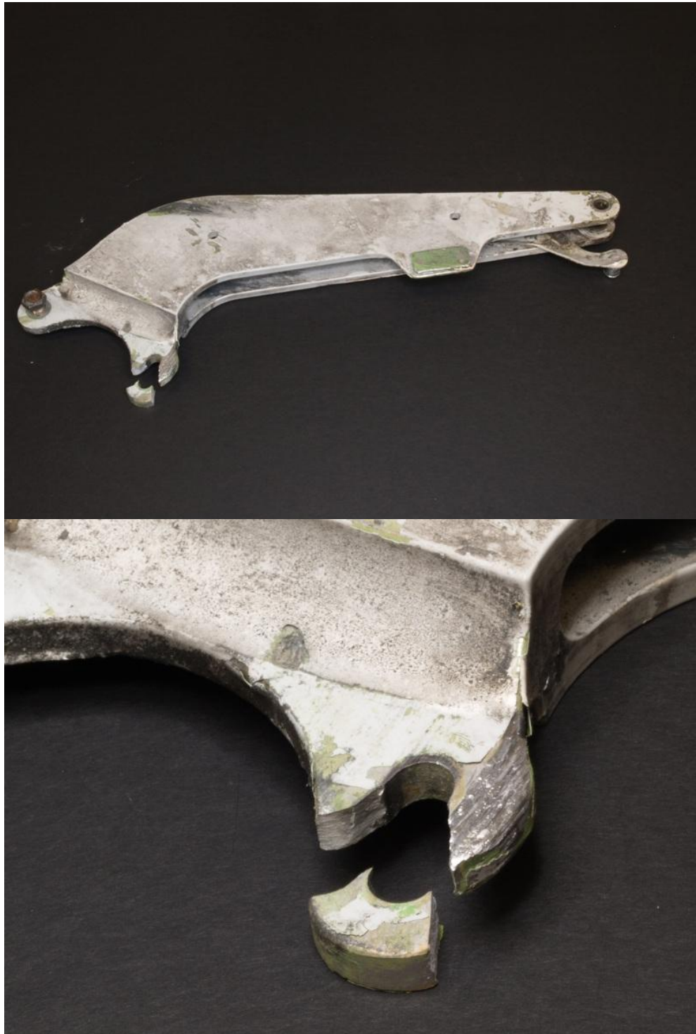
Figure 12. Inboard auxiliary track failure
