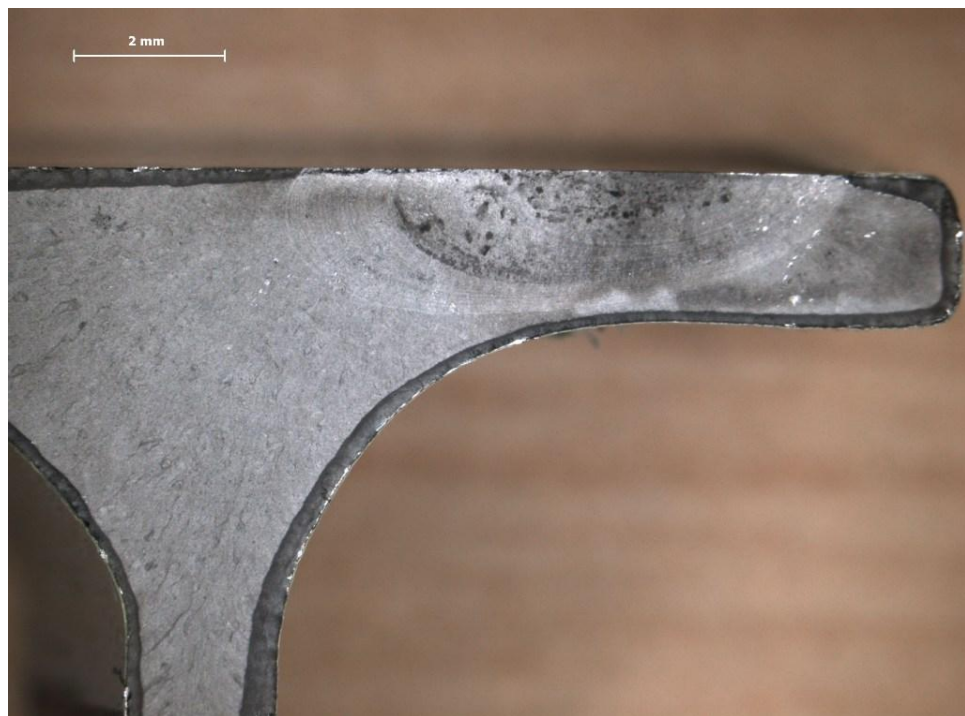
Figure 6. Fatigue region on lower flange exhibiting beach marks
