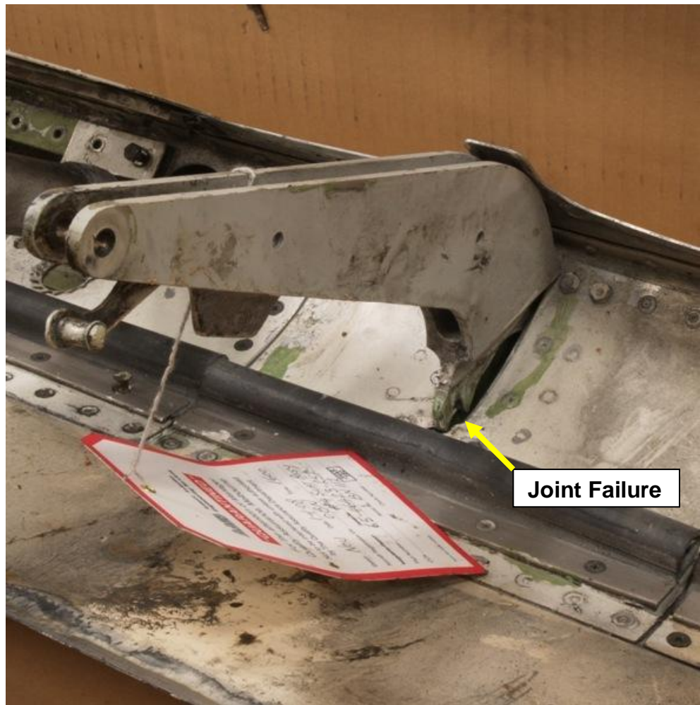
Figure 11. Inboard auxiliary track in situ
