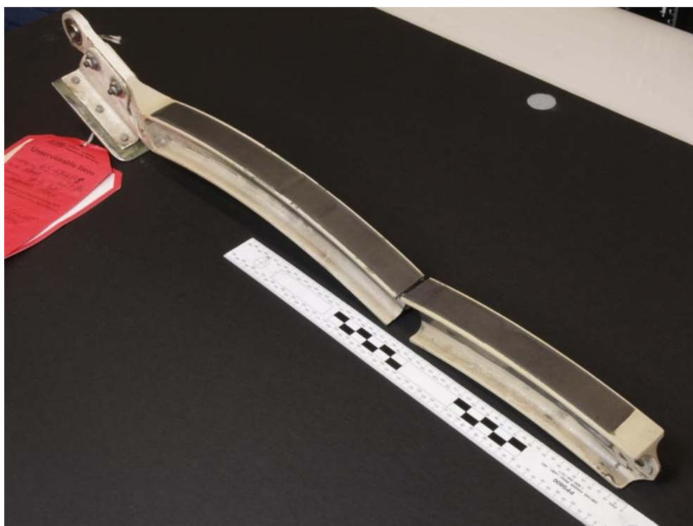
Figure 2. Failed inboard main slat track.
