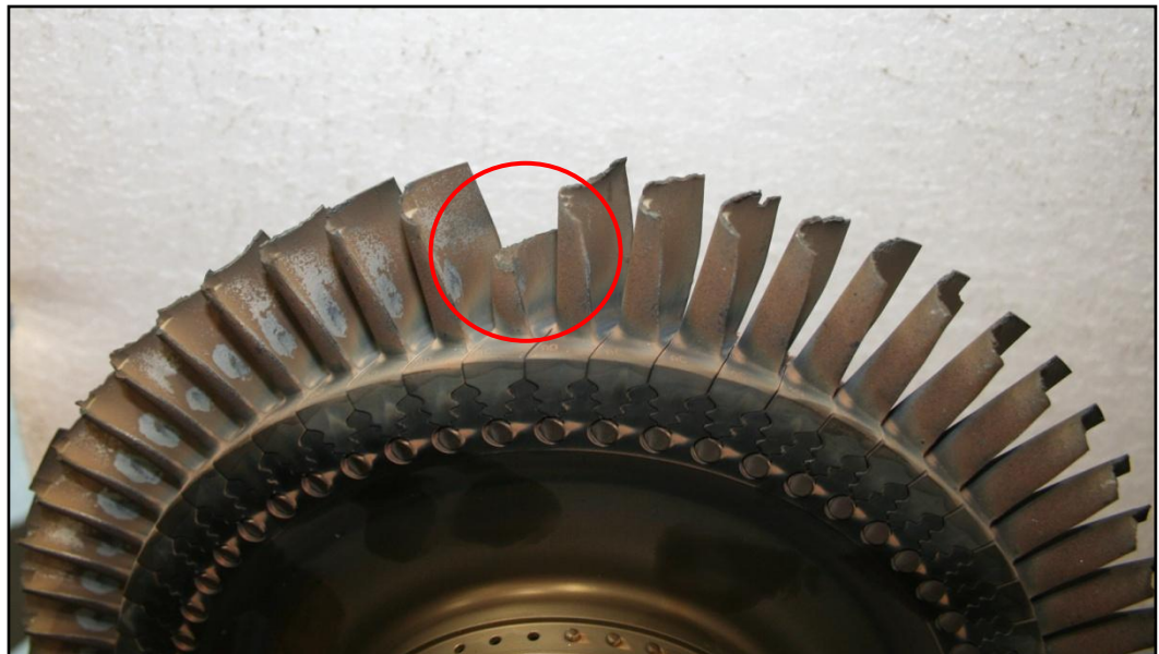
Figure 2: Severe CT blade tip erosion and fractured blade (circled)
