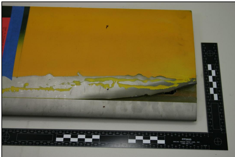
Figure 4: Main rotor blade 4225D showing the extent of skin separation on the underside of the blade
