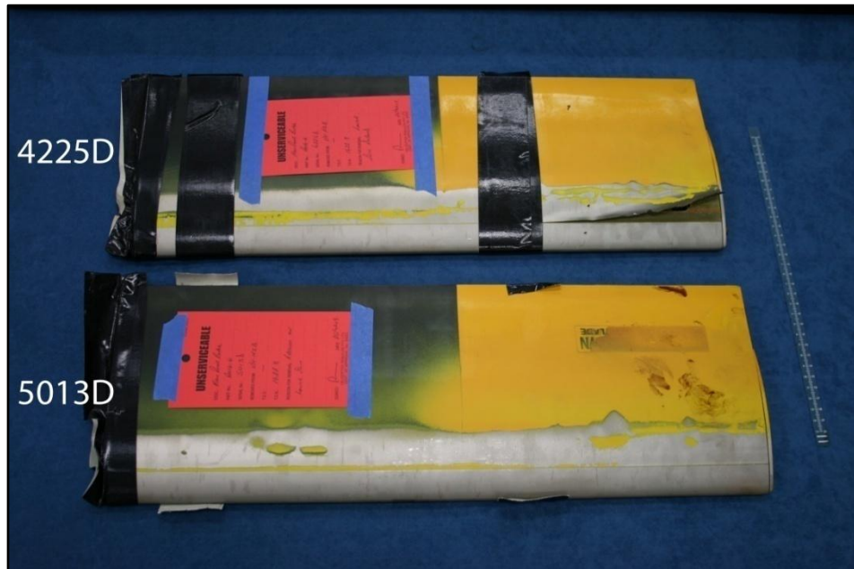
Figure 3: General view of the main rotor blade outer sections as received (underside)
