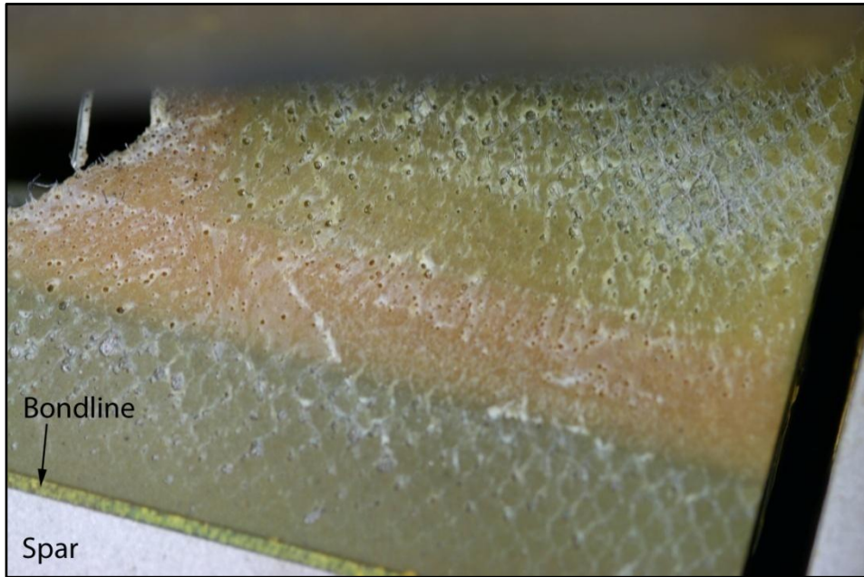
Figure 11: Magnified view of the bond line and adhesive surface immediately adjacent to the skin-to-spar bond line
