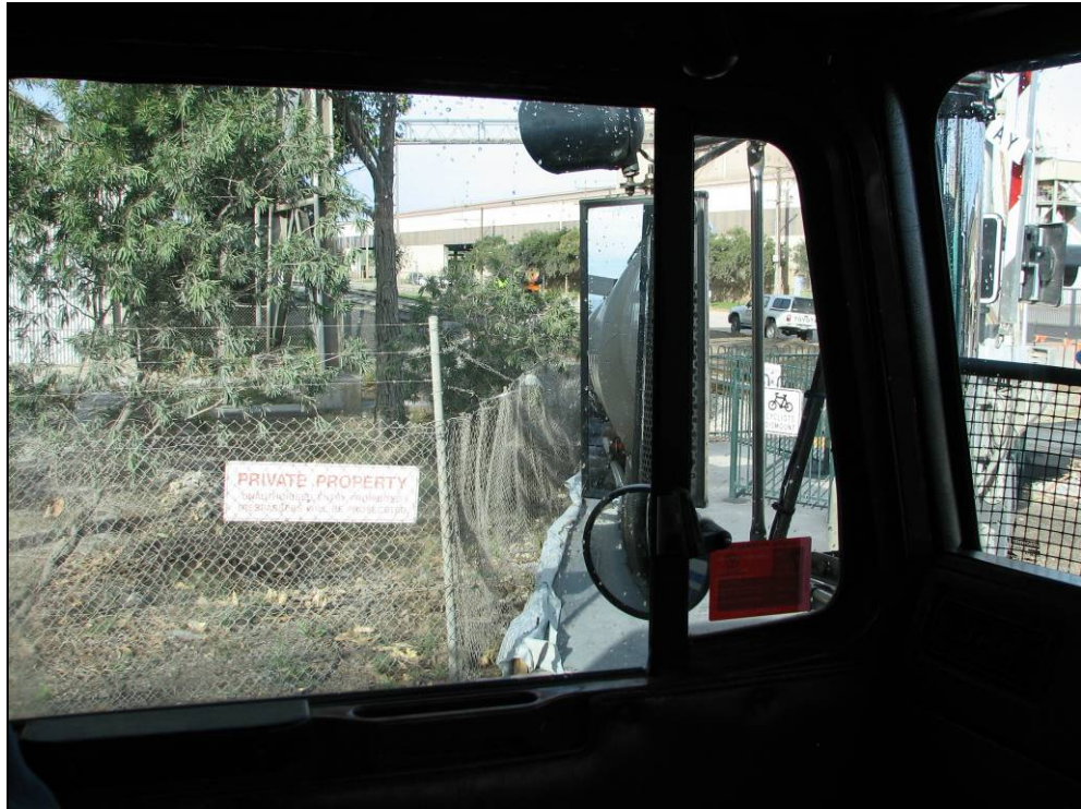
Figure 12: Visibility from prime-mover, nose 9.1 m from the nearest rail
