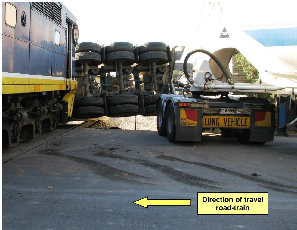
Figure 5: Tyre marks of rear bogie leading trailer
