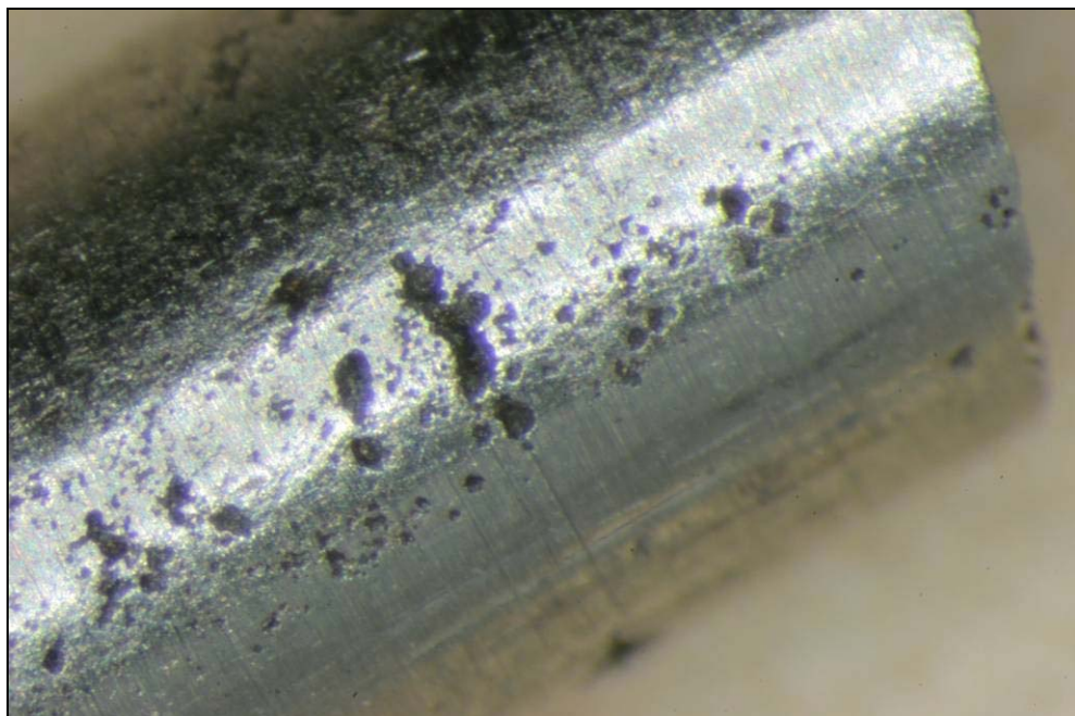
Figure 3: Pitted external surface of injector line
