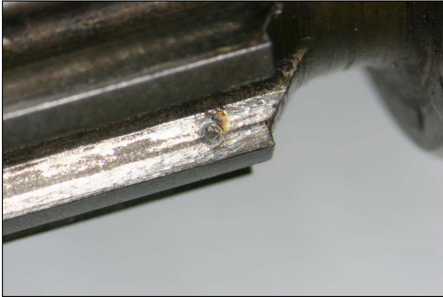
Figure 26: Pitting toward inner end of starter-generator drive spline
