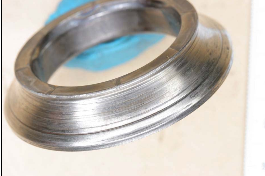
Figure 6: Rear section of the number-1 bearing inner race
