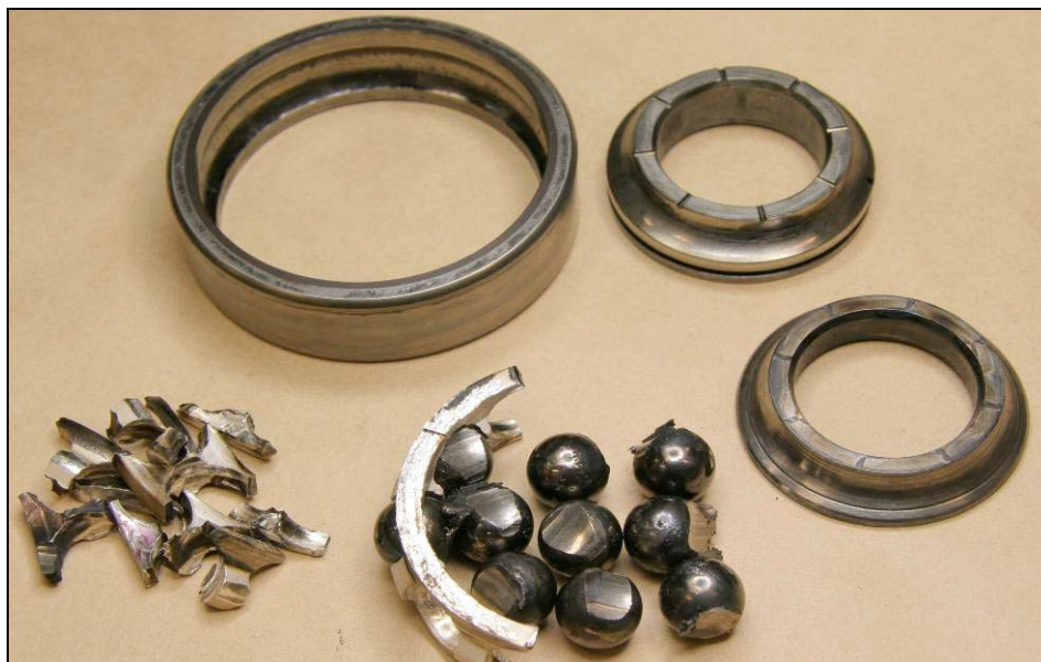
Figure 4: Failed number-1 bearing
