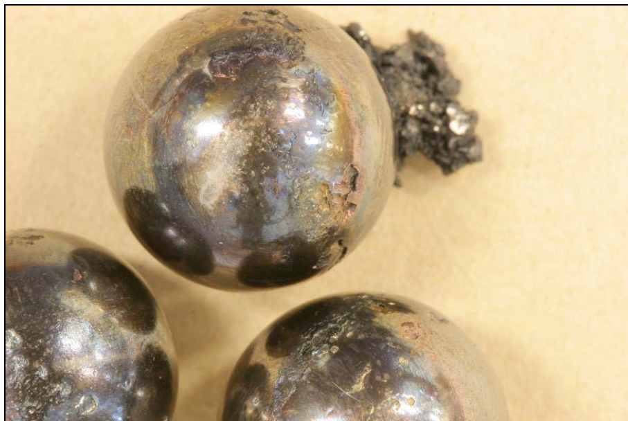
Figure 2: Rolling elements showing typical surface spalling damage
