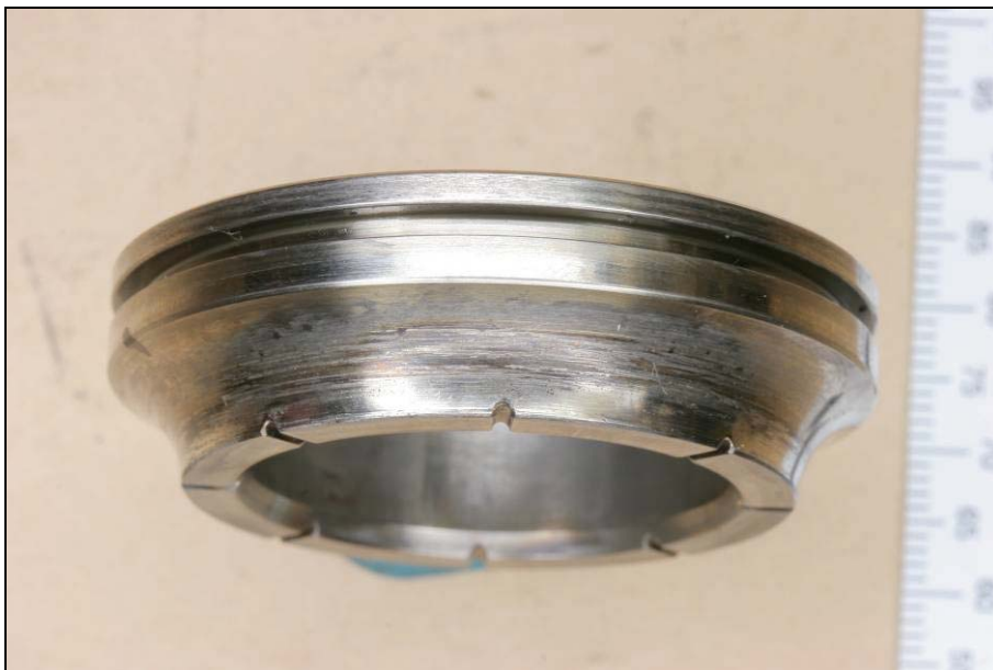
Figure 6: Rear section of the number-1 bearing inner race
