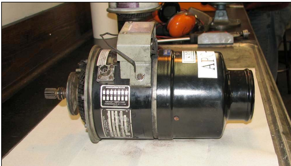
Figure 5: Failed starter-generator assembly
