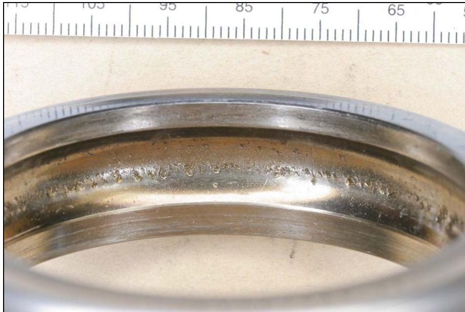
Figure 4: Atypical area on outer race surface (enclosed)
