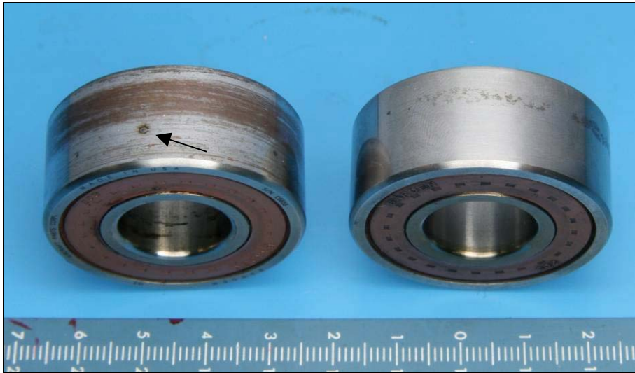
Figure 31: Typical pitting / re-melting damage as observed on the other accessory gear case components
