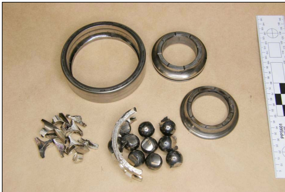
Figure 2: Rolling elements showing typical surface spalling damage
