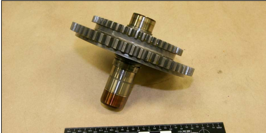
Figure 22: Prominent pitting and thermal tinting on a gear shaft tooth
