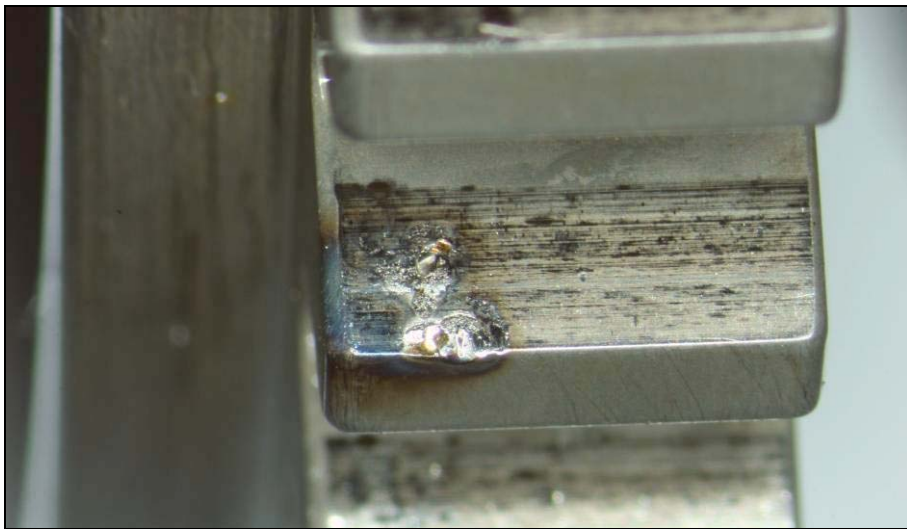
Figure 23: More pitting on the gear shaft teeth – adjacent to the area shown in Figure 22
