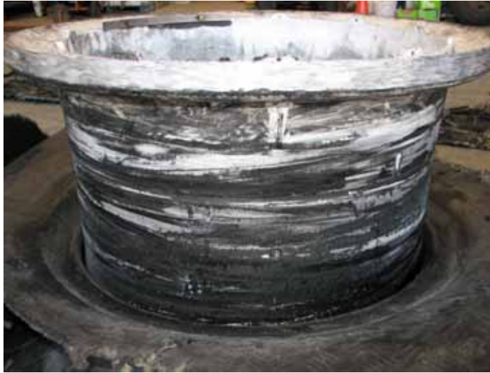
Figure 2: Damaged number-1 wheel assembly
