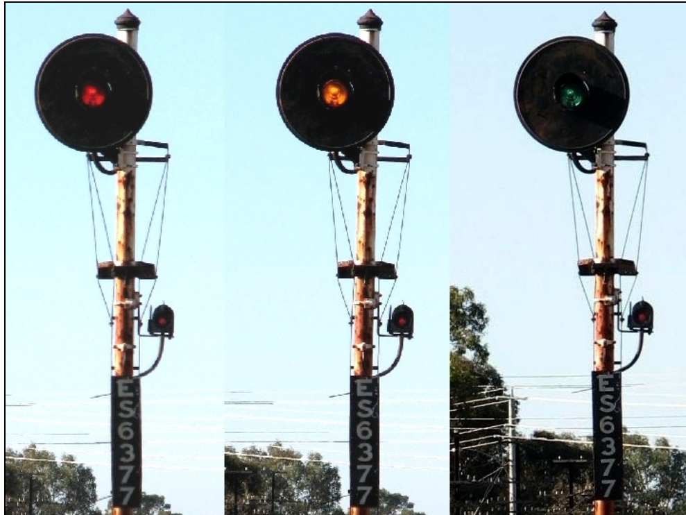
Figure 25: Signal ES6377, top arm showing the 'red', 'yellow' and 'green' aspects.
