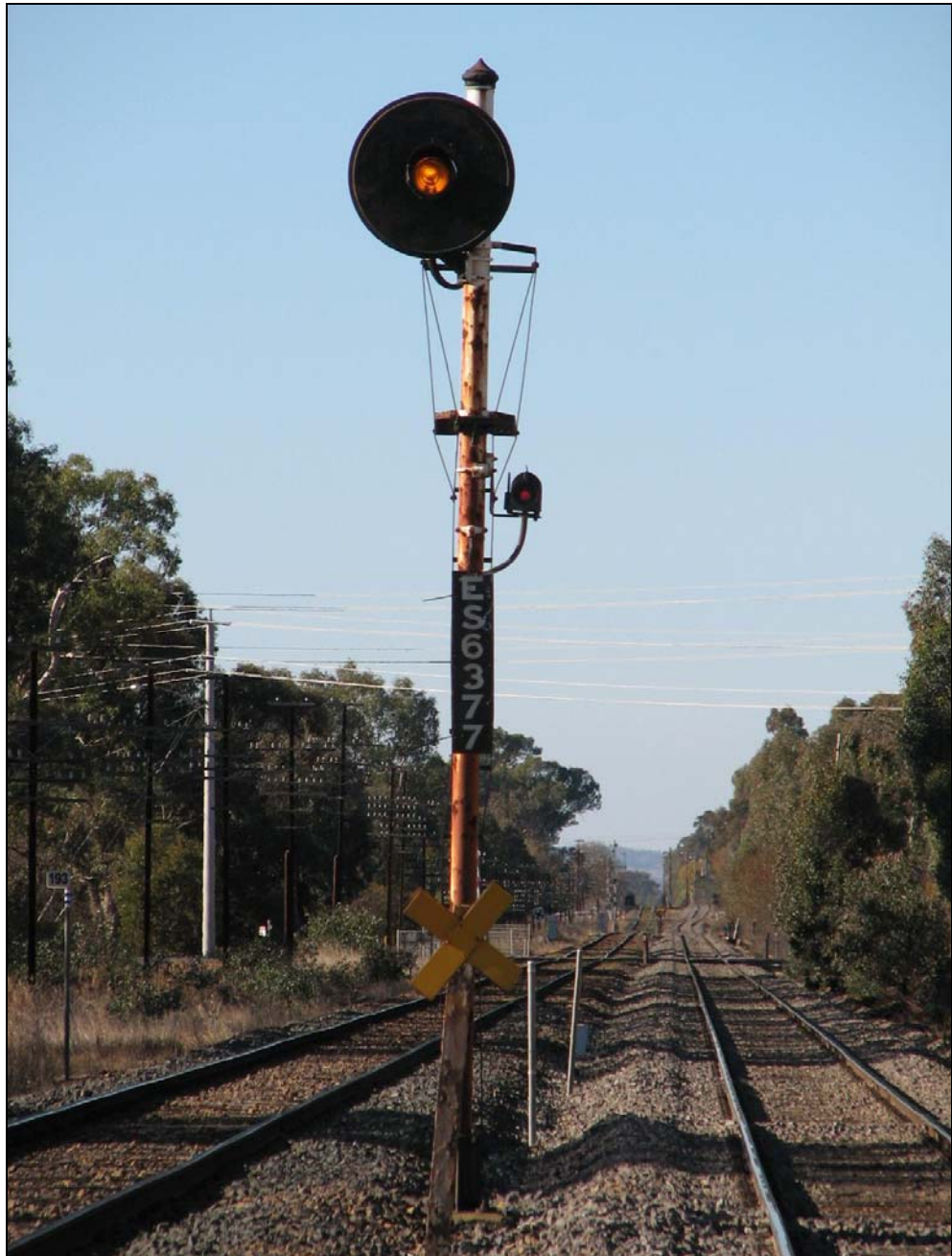
Figure 14: Outer signal No. ES6377 looking towards Benalla. ES6377 is a three aspect signal. Top arm as shown is displaying 'Normal Speed Proceed – Yellow Aspect'
