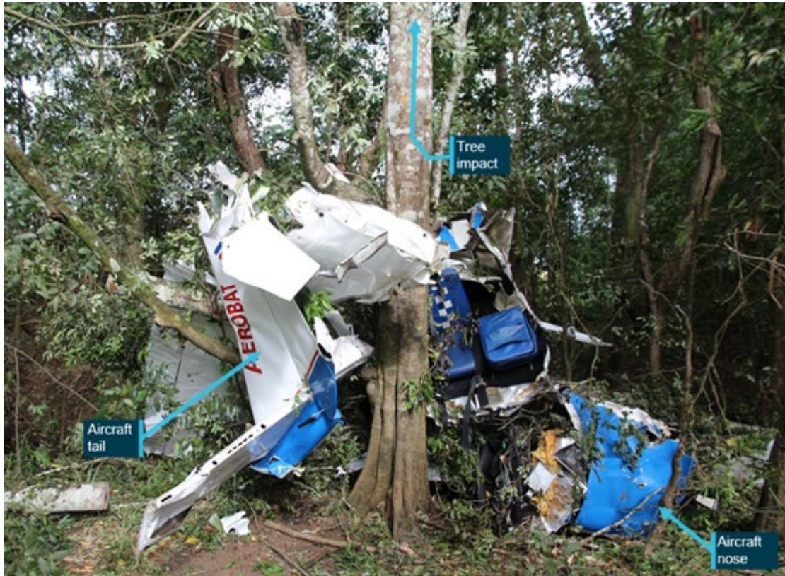
Figure 8: Aircraft main wreckage at the base of a large tree that was struck
