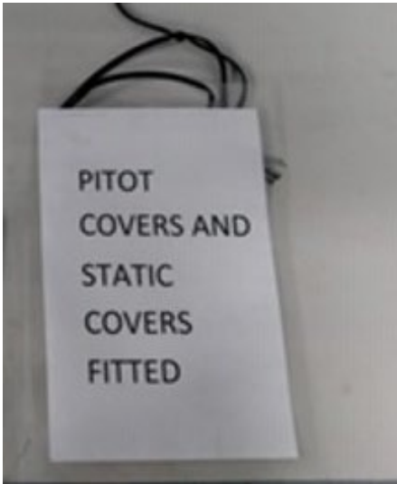
Figure 4: Control column warning placard
