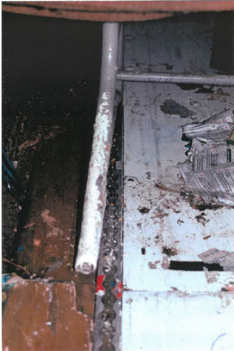
Figure 3: Deformation of the rear portion of the seat frame.
