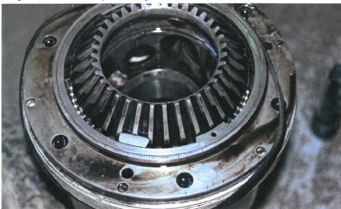
Figure 1: The vernier scale on the outside cam with feather stop giving blade pitch angle of 65 - 66°.
