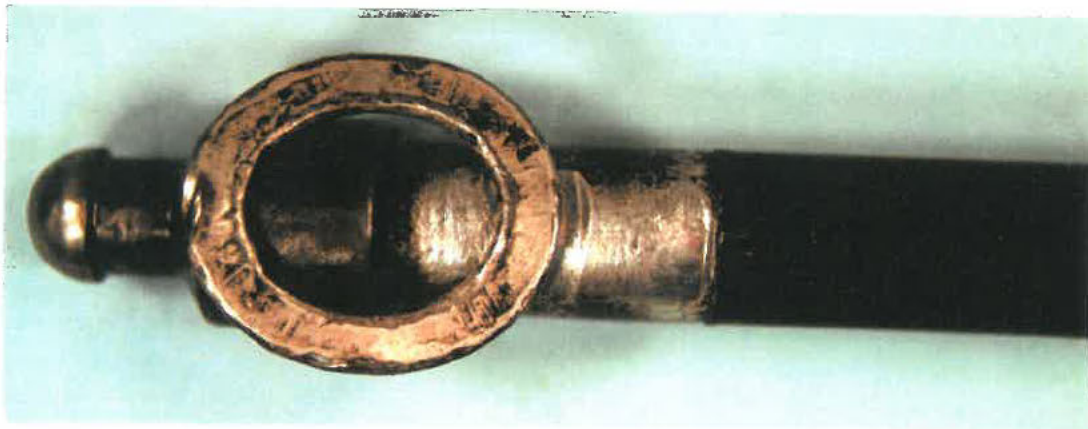
Figure 7: Deformed washer and deep rub marks on the push rod.
