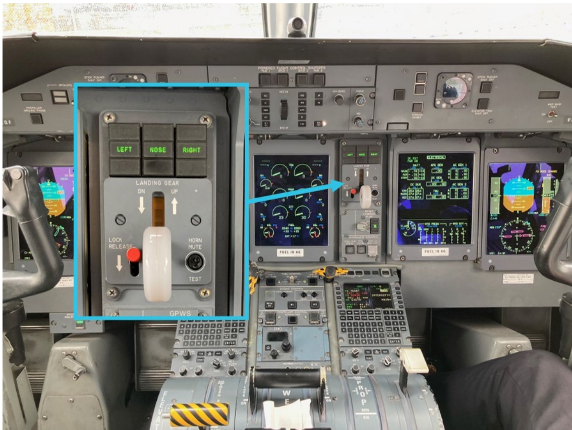
Figure 1: Landing gear handle and advisory panel
