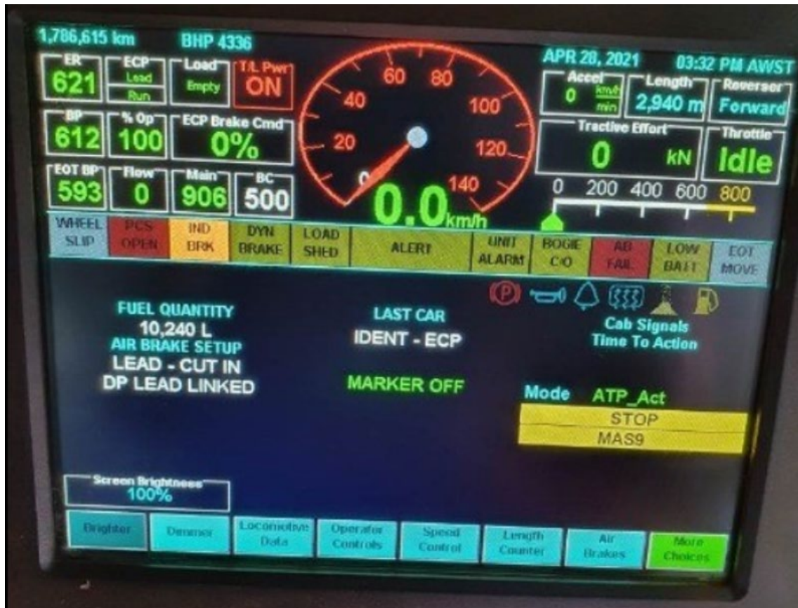
Figure 6: Typical FIRE system display
