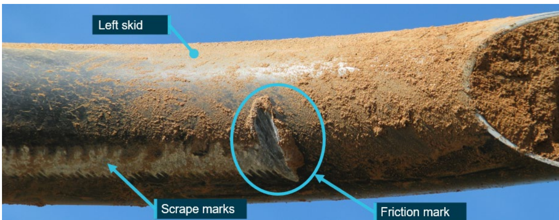
Figure 3: Wire marks on VH-HNF’s left skid
