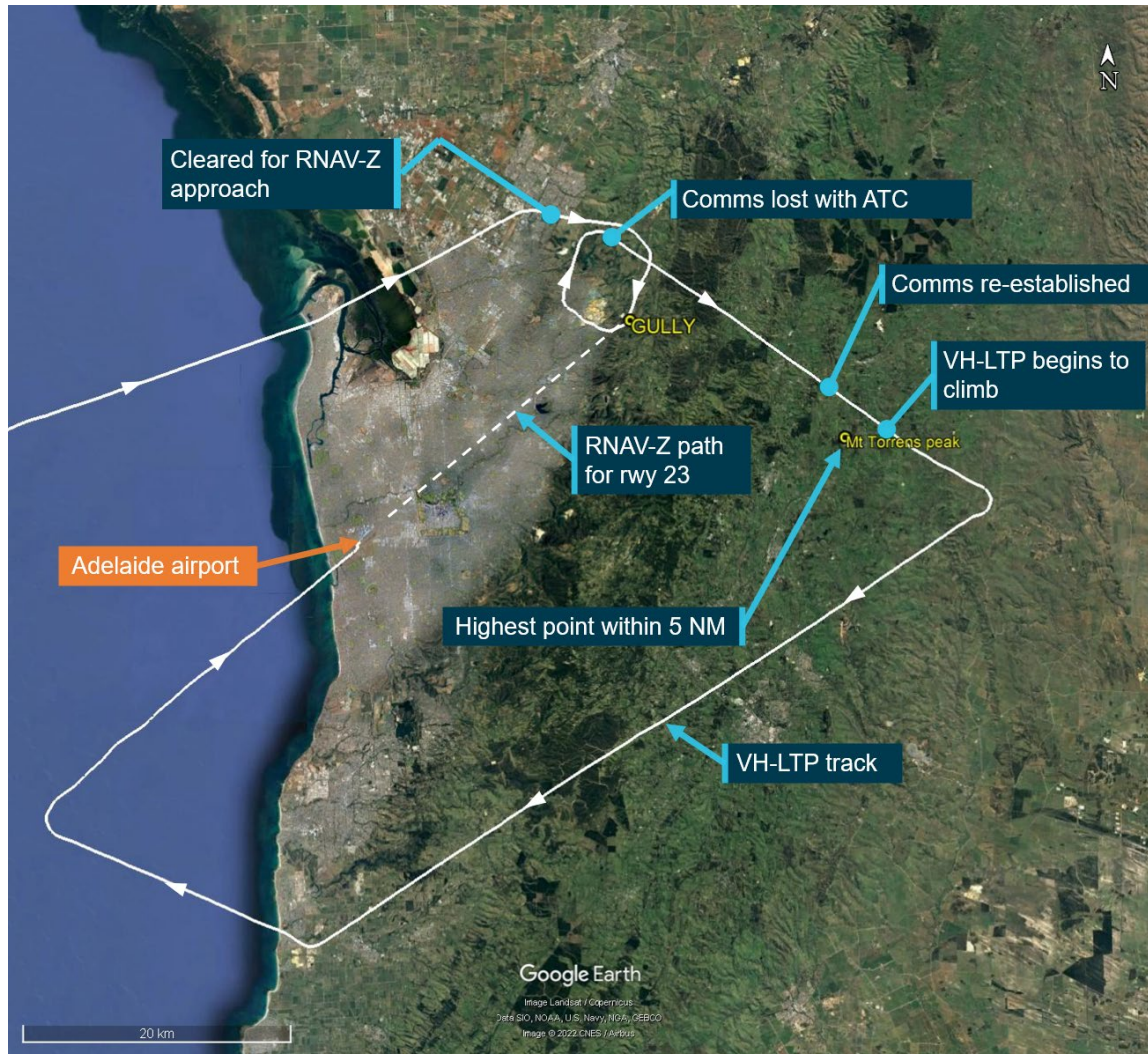
Figure 1: VH-LTP flight path (dotted line shows RNAV instrument approach path)
