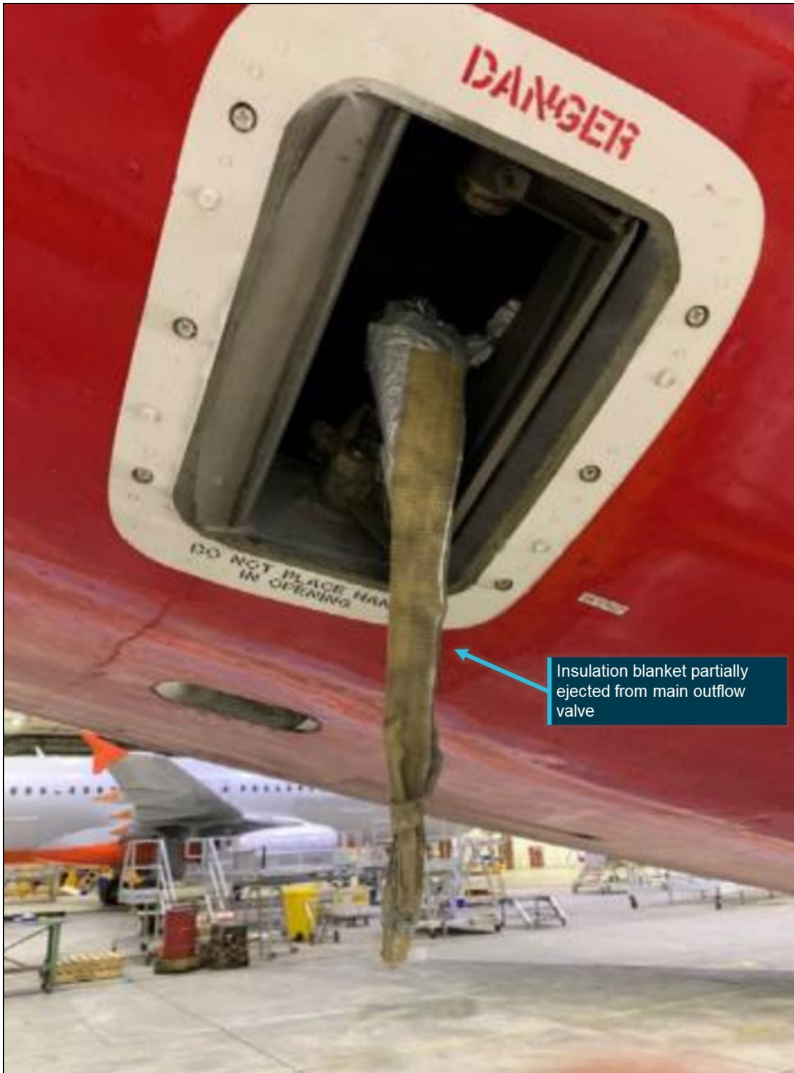
Figure 3: Main outflow valve after occurrence
