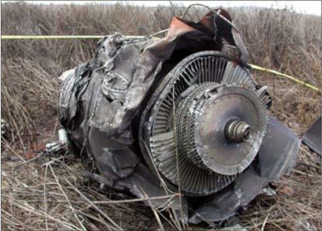
FIGURE 17: Typical engine damage
