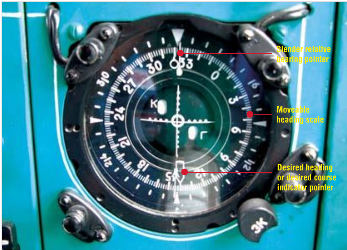
FIGURE 9: Course indicator similar to those fitted in the occurrence aircraft
