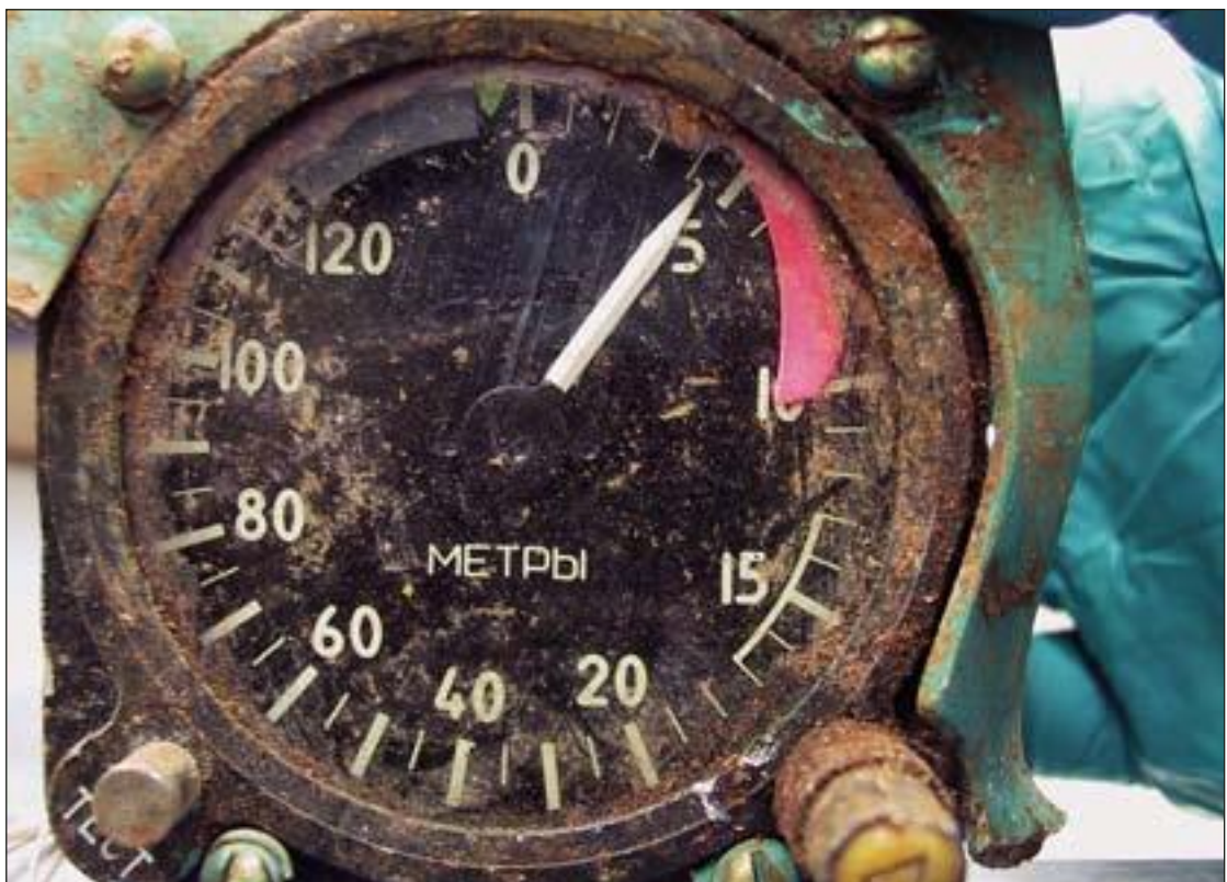
FIGURE 25: The PB-150 radio altimeter indicator located in the aircraft wreckage
