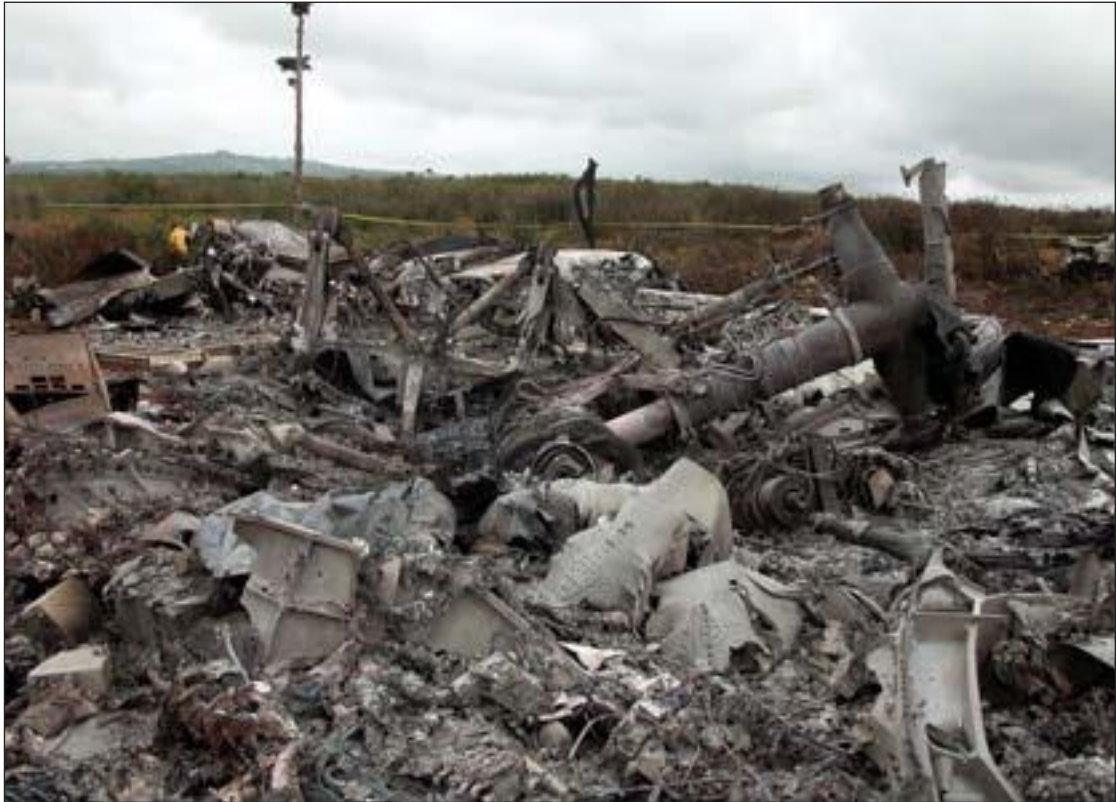
FIGURE 28: Fire damage in main wreckage area
