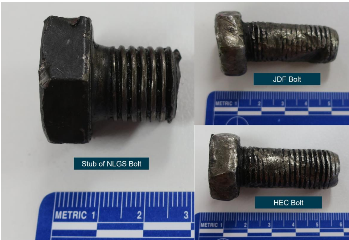
Figure 6: Side view of three axle end cap bolts, including broken NLGS bolt
