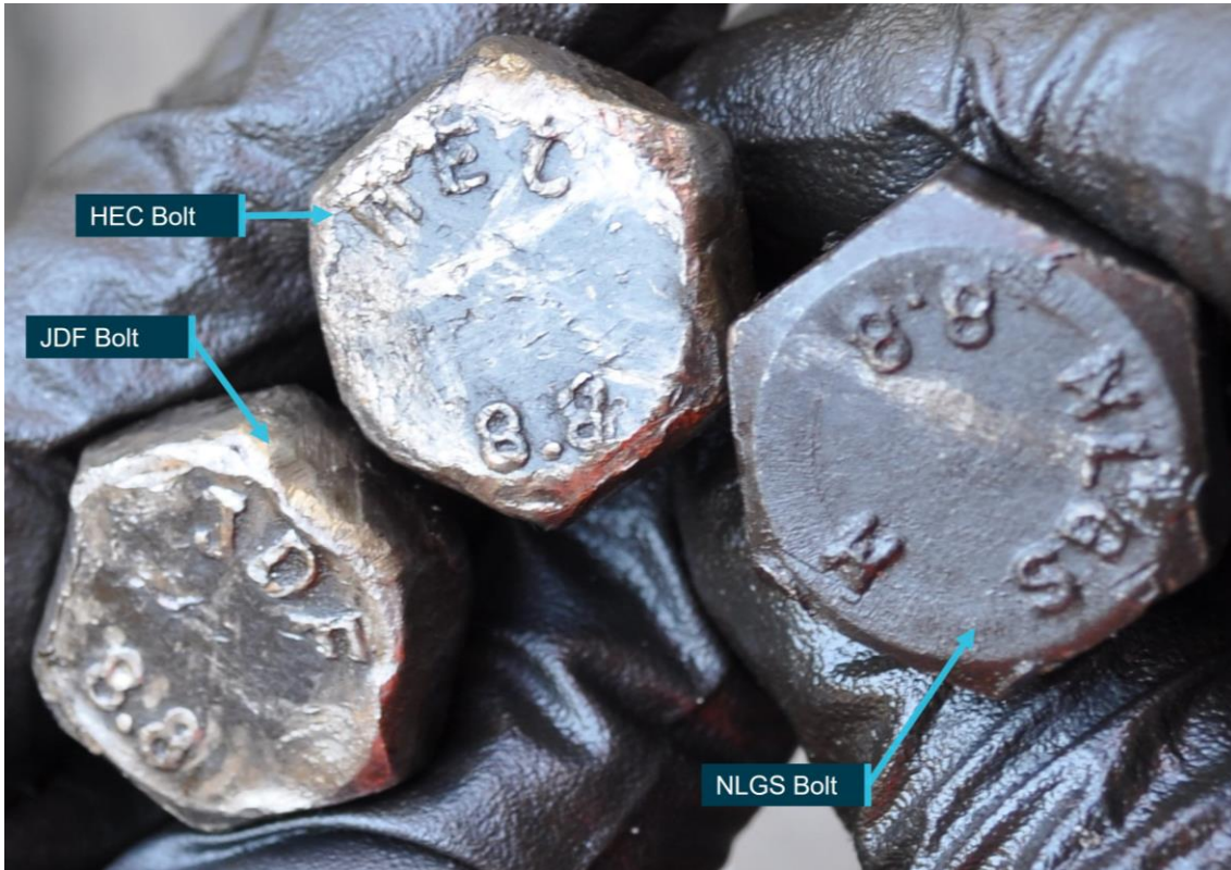
Figure 5: Three types of axle end cap bolts removed from hub following incident
