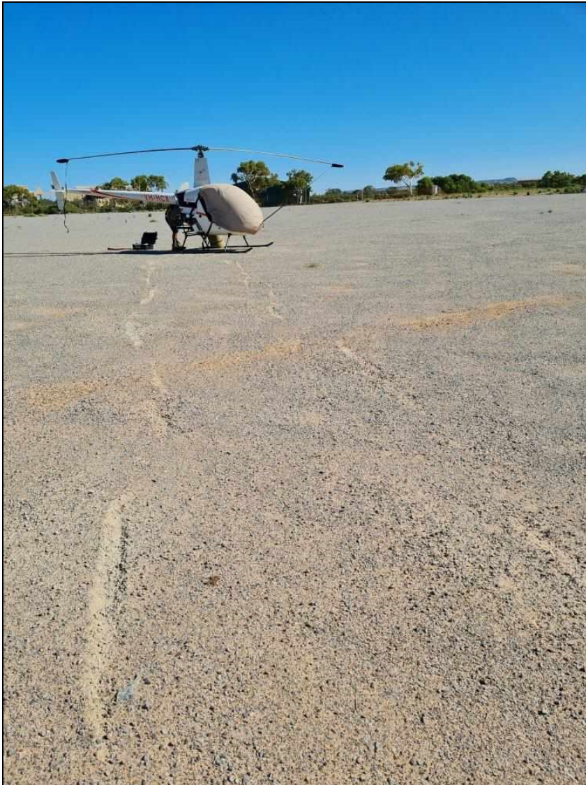
Several heel-toe skid marks were created during the landing. The helicopter subsequently yawed right after the pilot attempted to reposition the helicopter. Source: Fortescue Helicopters
