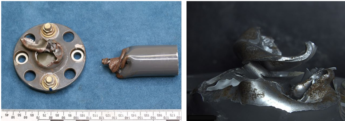
Figure 4: Gross ductile twisting and overstress fracture of the drive shaft
