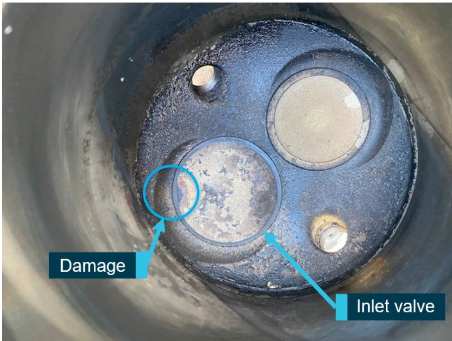
Figure 3: Internal view showing localised heat damage to the inlet valve from the number-four cylinder of the engine
