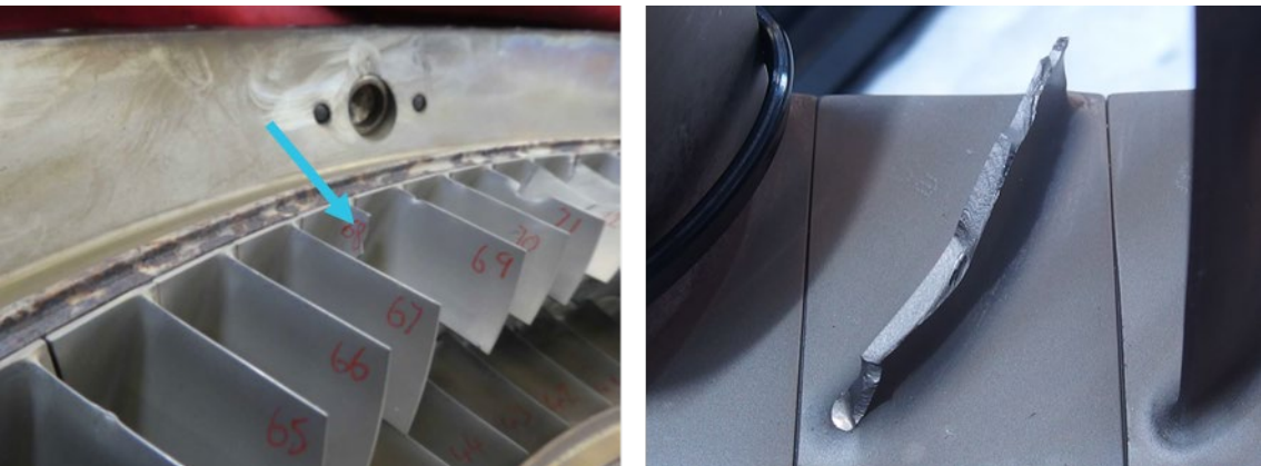
Figure 6: Stage 6 vane fatigue failure
