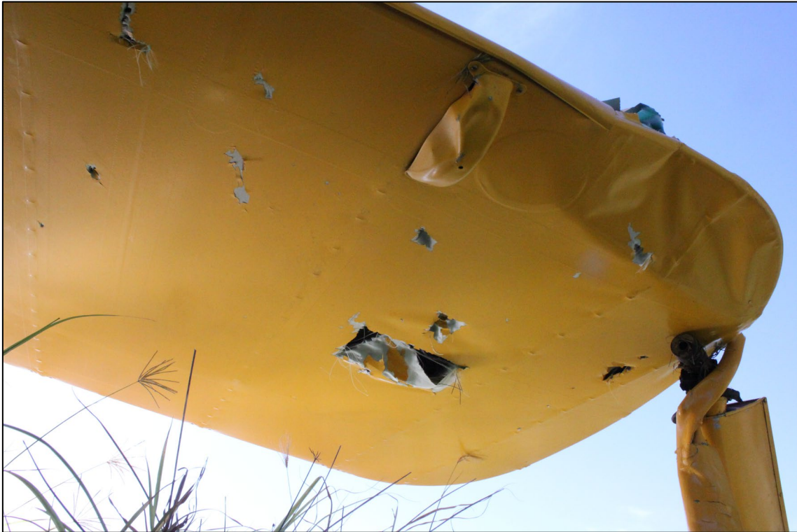
Figure 4: Tree impact marks on underside of upper left wing
