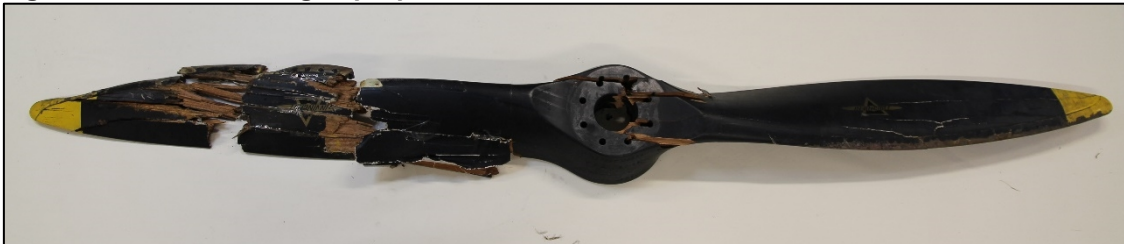
Figure 5: VH-UZB damaged propeller
