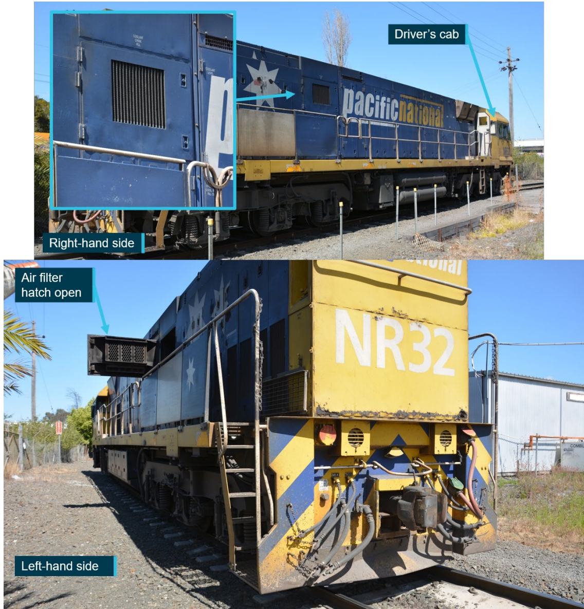
The right-hand and left-hand sides of an NR locomotive are shown. The left-hand side of the locomotive is shown with the air filter hatch open and protruding past the body of the locomotive (rolling stock outline). Source: OTSI
