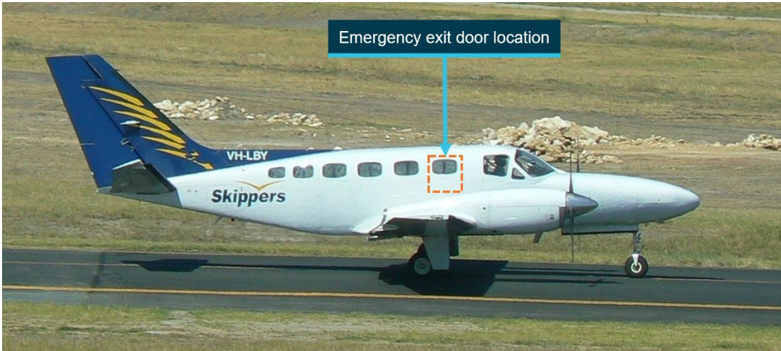
Figure 2: VH-LBY and the location of the emergency exit door
