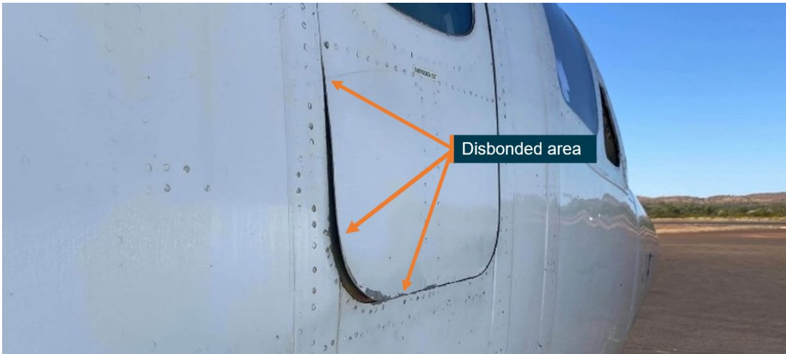
Figure 3: Separation of the emergency exit door outer skin
