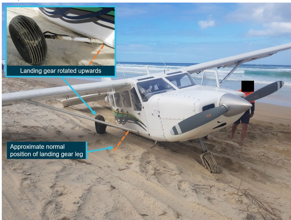
Figure 1: VH-BFS where it came to rest on 24 August, showing the right landing gear collapsed
