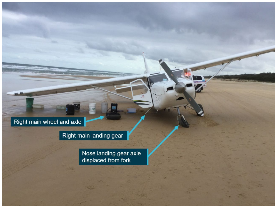
Figure 2: VH-BFS where it came to rest on 31 October, showing the right main wheel separated from the aircraft
