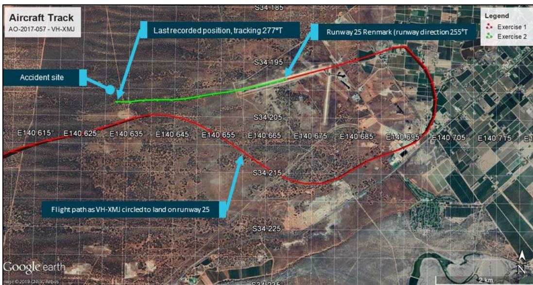
Figure 1: Position information of VH-XMJ as the aircraft circled and landed on runway 25 (depicted in red), before backtracking and departing (depicted in green).
