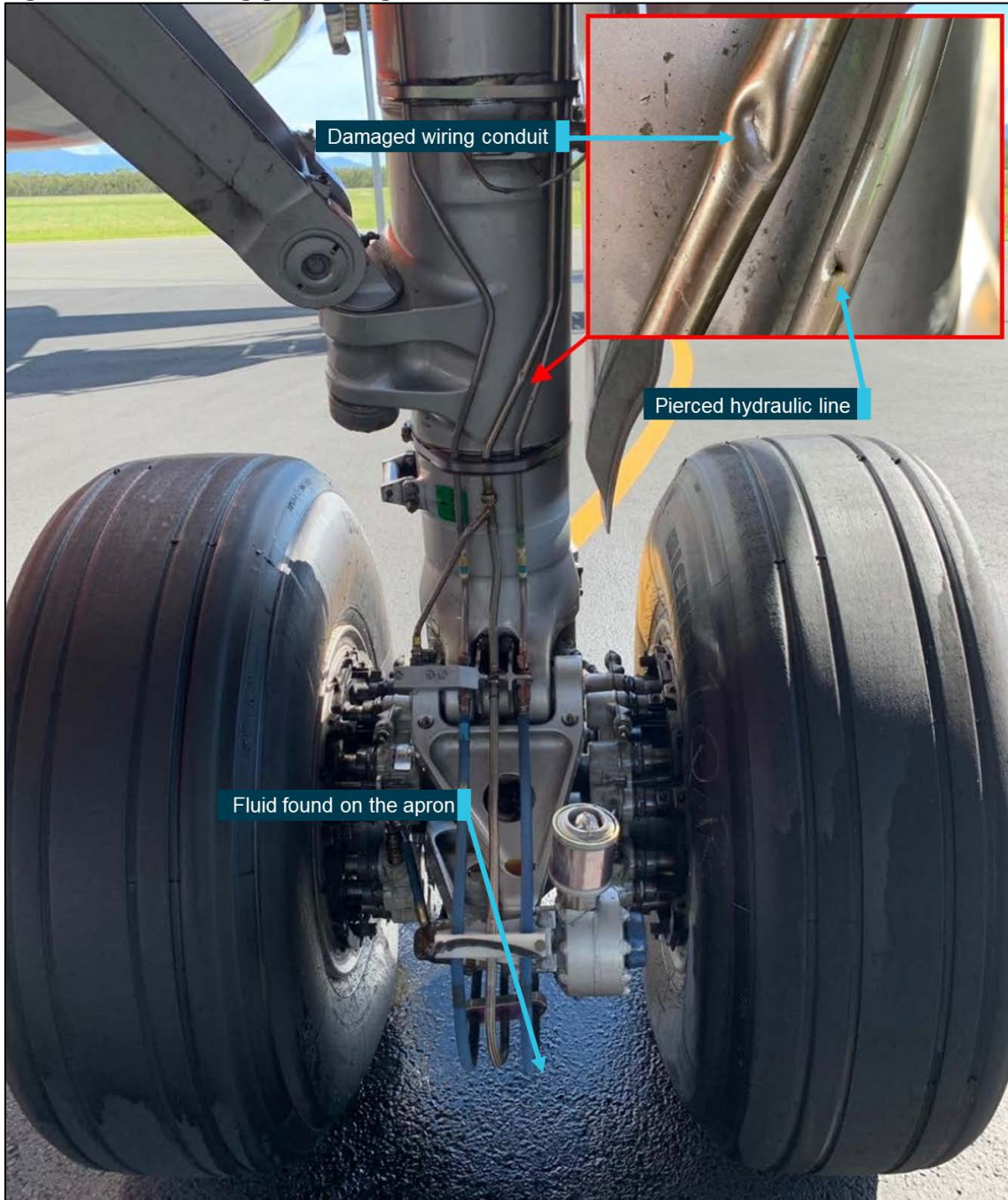
Figure 2: Main landing gear damage
