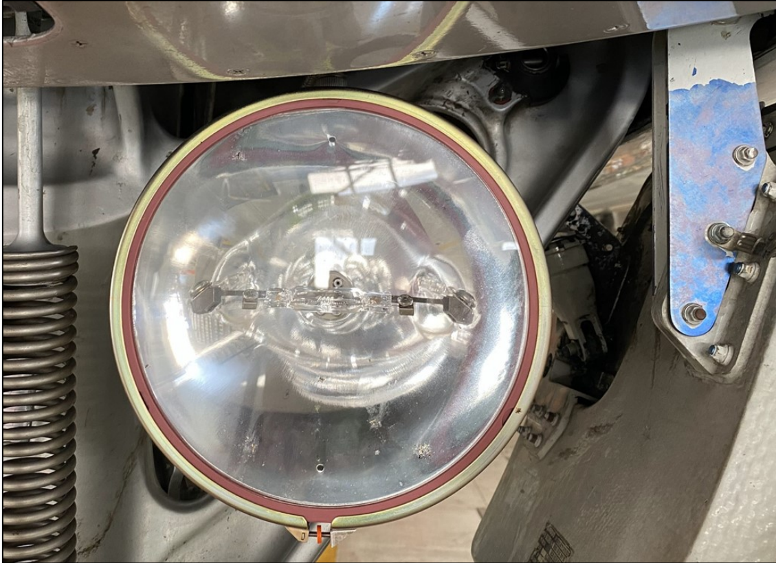
Figure 3: Undamaged nose gear landing light with polycarbonate cover
