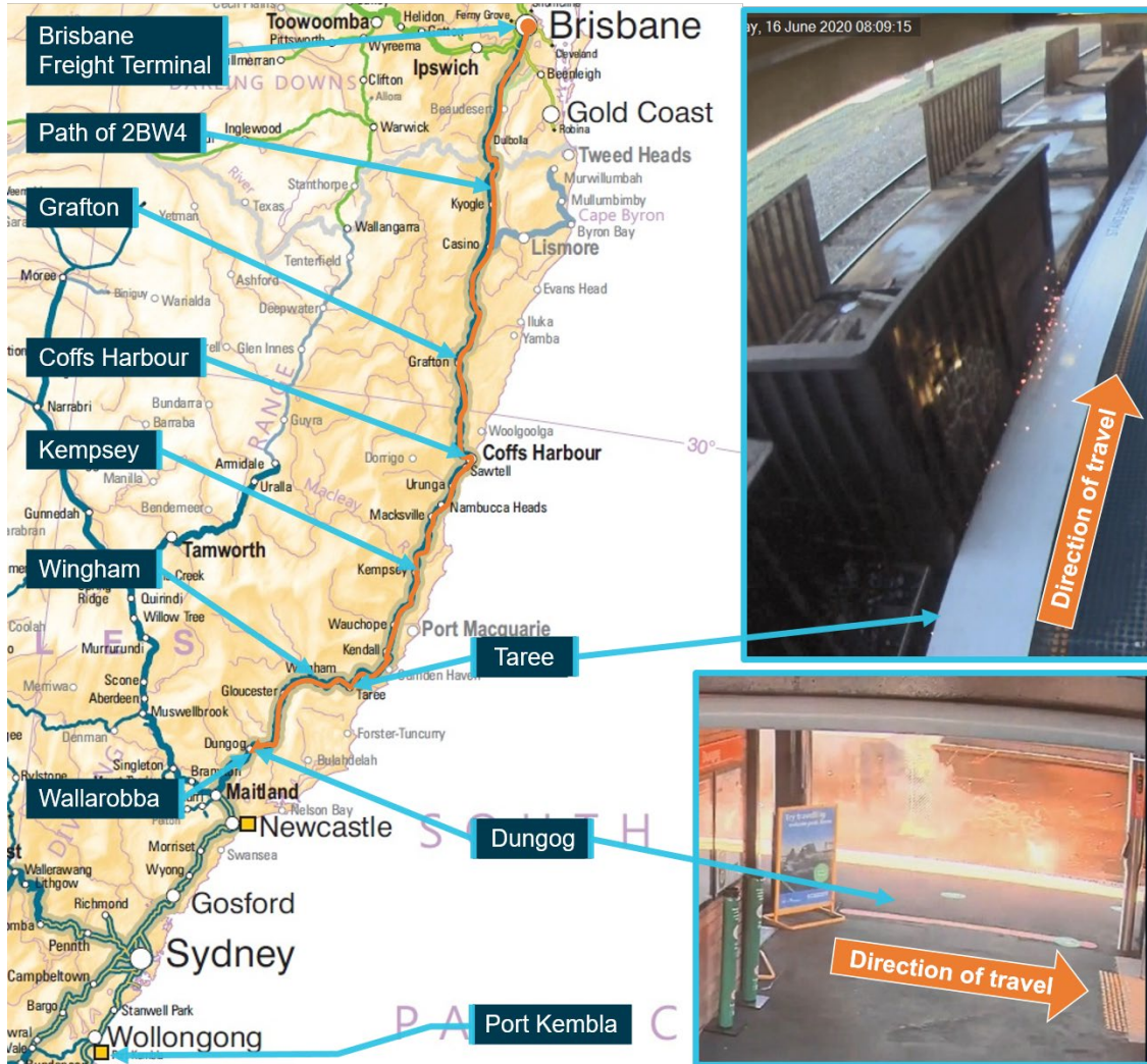
Map showing the path of train 2BW4 and platform locations. Footage from Taree and Dungog platforms inset showing wagon RKOX4055Y contacting the platforms.
