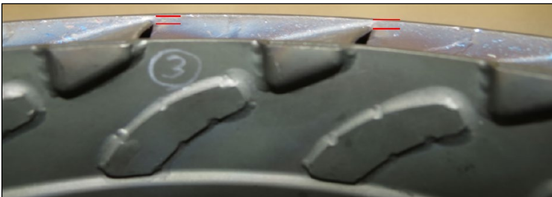
Figure 15: Trailing edge positioning variations against the outer shroud from the STI-repaired CT vane ring, highlighting a non-conformance
