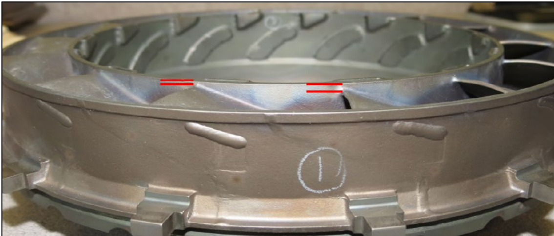
Figure 14: Trailing edge positioning variations against the inner shroud from the STI-repaired CT vane ring, highlighting a non-conformance
