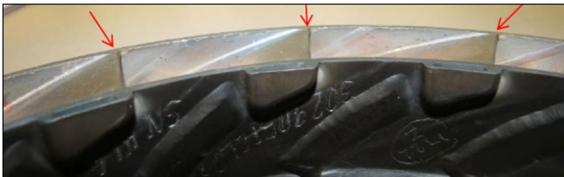
Figure 16: Example of trailing edge positioning against the outer shroud from a PWC-manufactured CT vane ring
