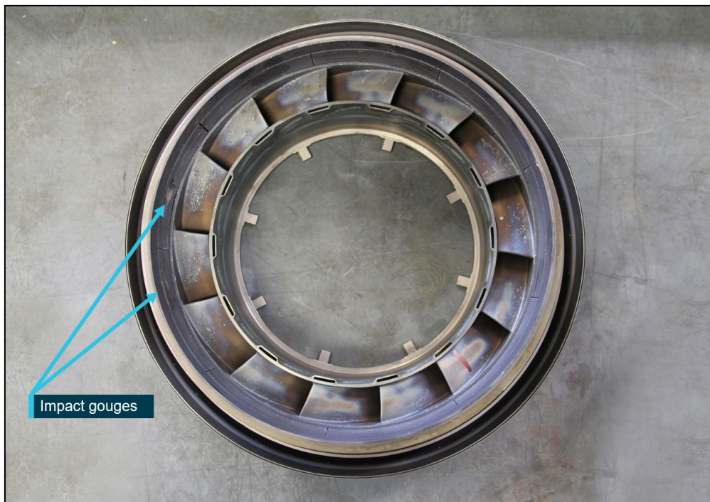
Figure 10: Compressor turbine vane ring assembly, view of the downstream face with gouge damage (labelled)
