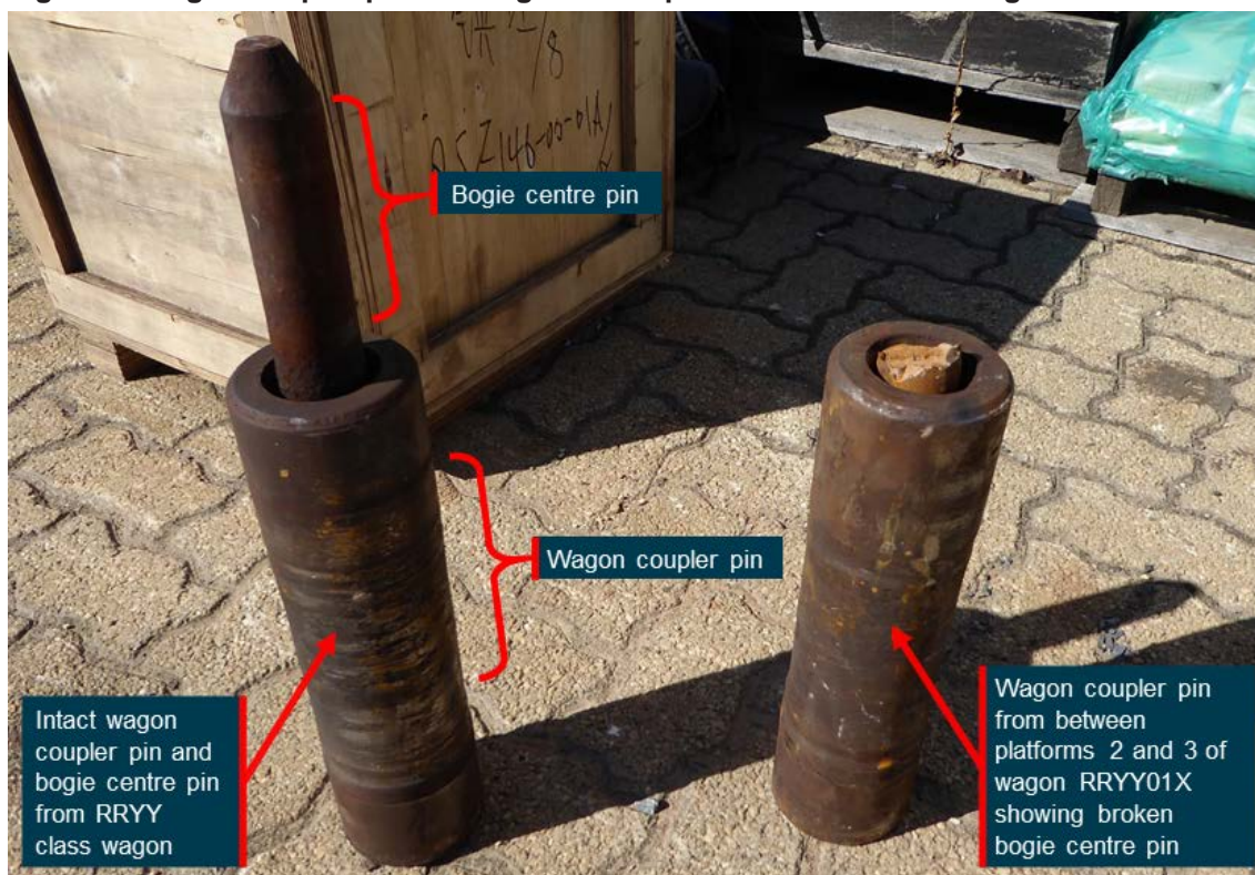
Image shows an intact combined wagon coupler-pin and bogie centre-pin from a RRYY class wagon, alongside the wagon coupler-pin from wagon RRYY01X with missing bogie centre-pin. Source: ATSB
