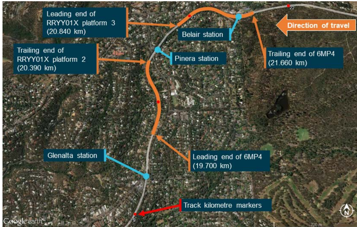
Figure 6: The stopped location of both portions of 6MP4 after the train separated
