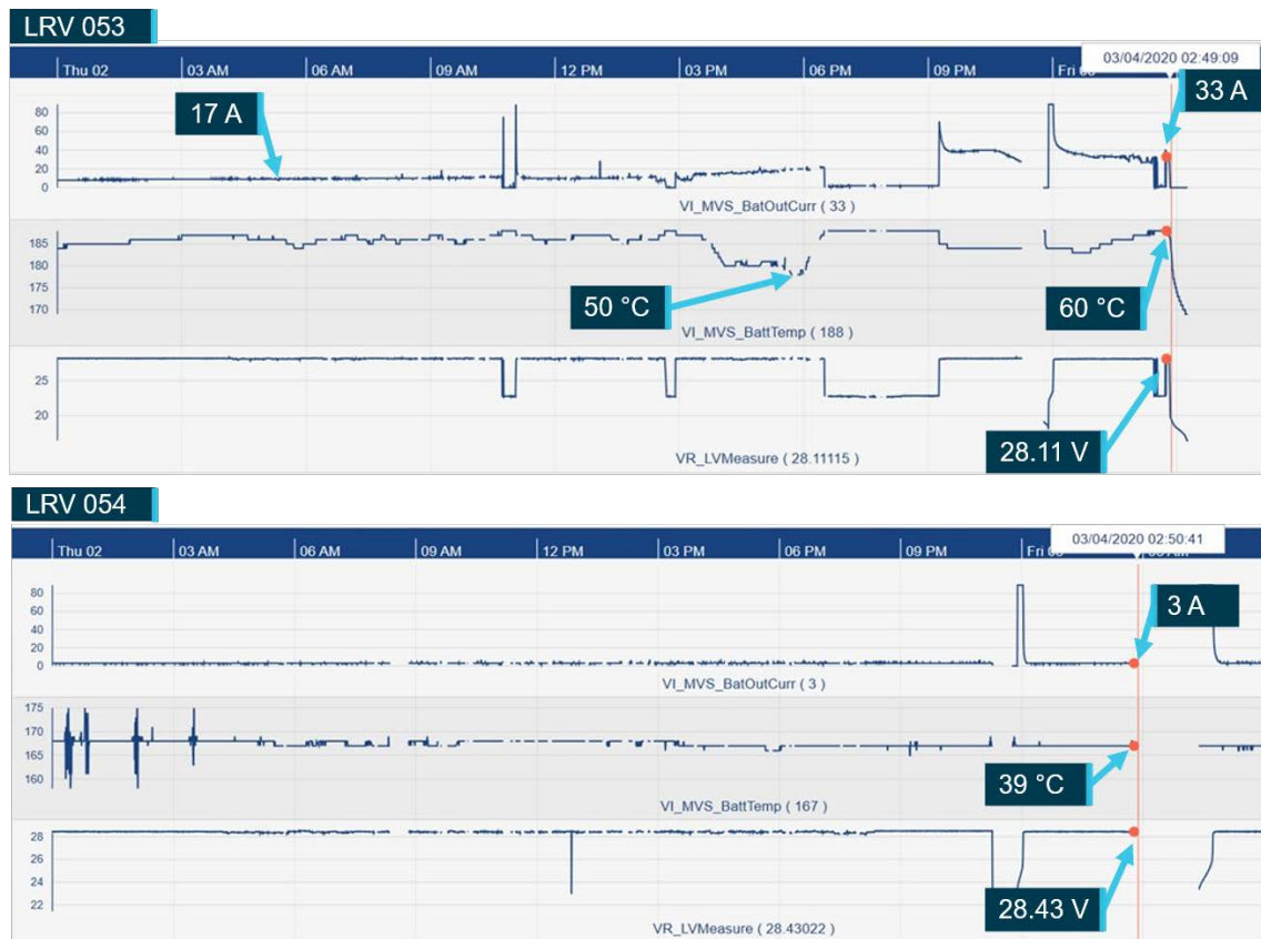
Figure 8: LRV 053/054 battery charging data from 2 and 3 April 2020
