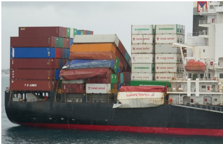
Figure 5: Damaged containers in bays 52 and 56
