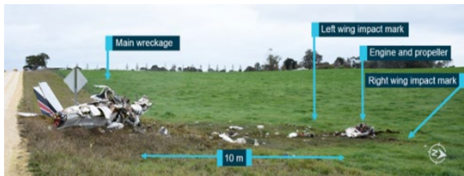
Figure 1: Accident site, showing the engine and propeller location, the left and right wing impact marks and the main wreckage
