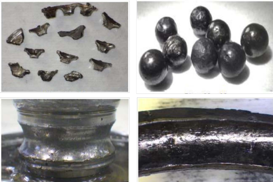
Figure 1: No. 30 bearing broken cage pieces, damaged ball bearings and spalling on the inner and outer bearing races
