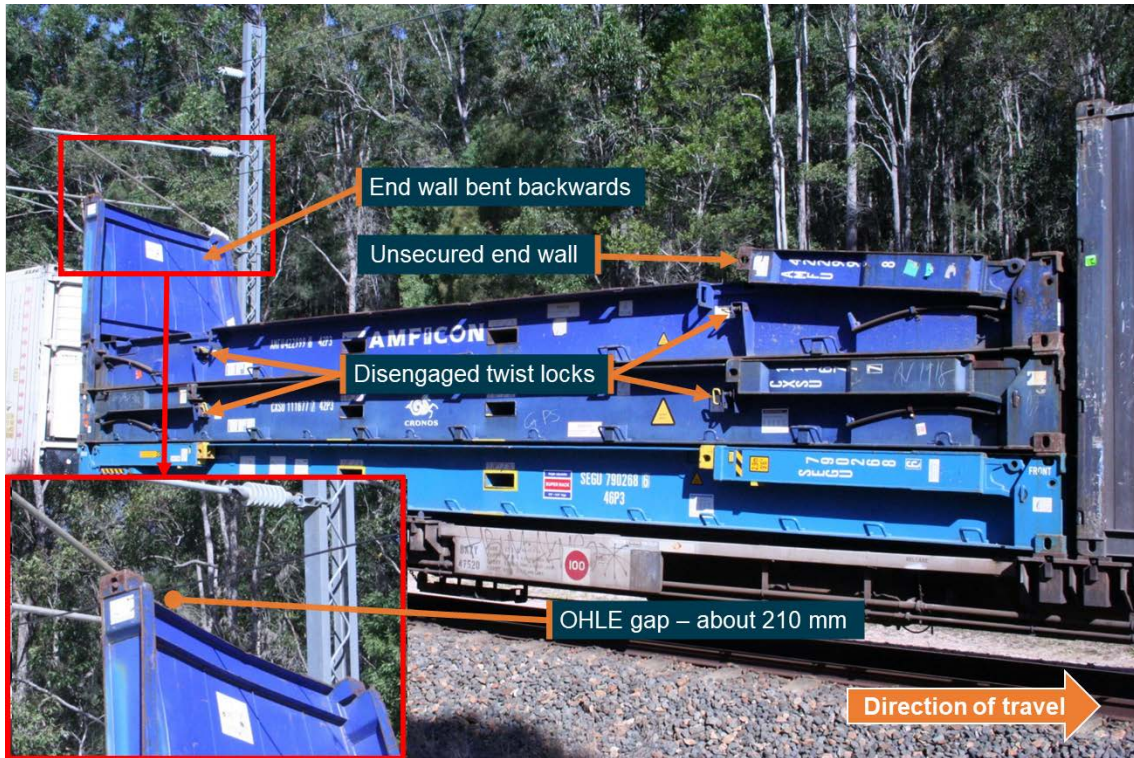
Image shows the extended end wall of the top nested flat rack, loaded on wagon BAZY 47520. The distance between the end wall and the OHLE contact wire is about 210 mm.
