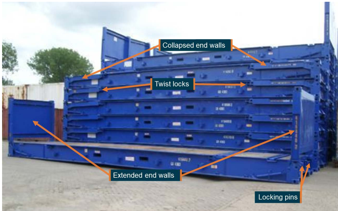
Figure 8: Flat rack containers
