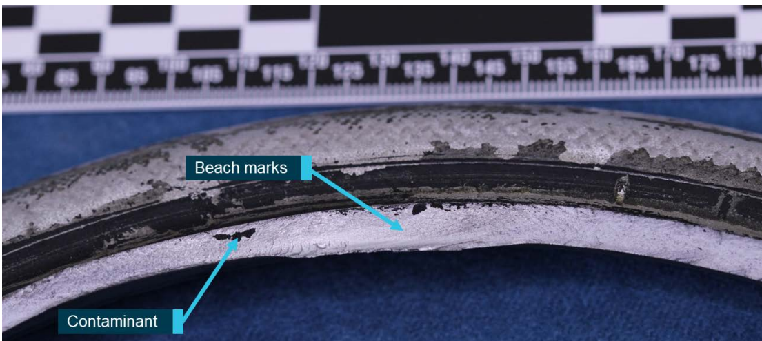
Figure 4: Magnified view of fatigue area showing crack progression along the bead seat and evidence of tyre contamination on the fracture surface
