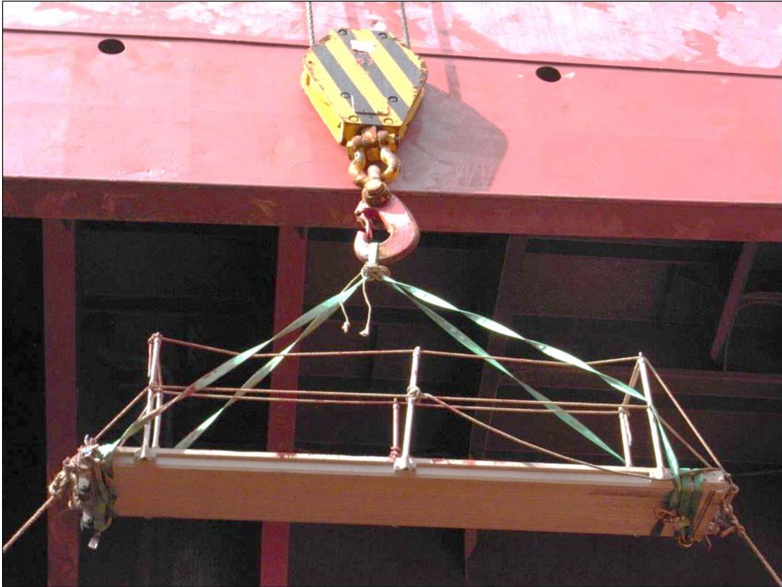
Figure 8: Re-enactment of the approximate location of the platform and falling block at the time of the accident
