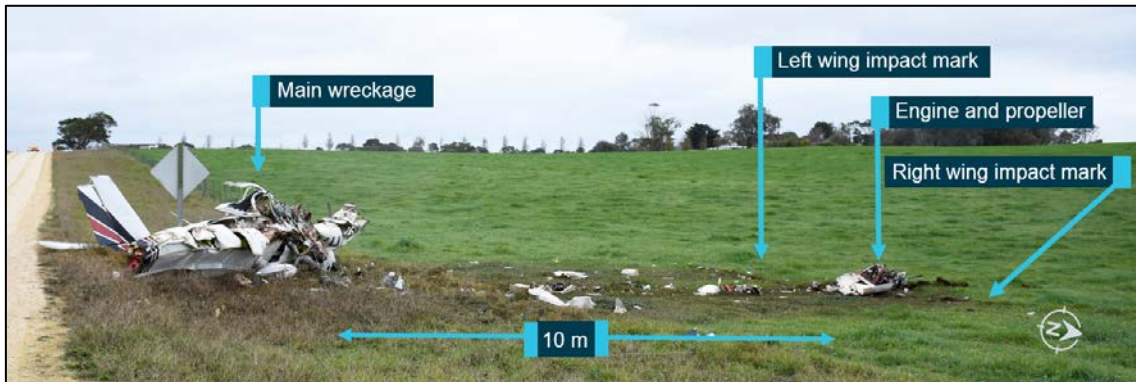
Figure 4: Accident site, showing the engine and propeller location, the left and right wing impact marks and the main wreckage
