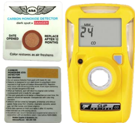
Passive chemical spot detector as carried in VH-NOO (L) with example BWC2R-M1025 active digital CO detector (R) (Source: ATSB)
