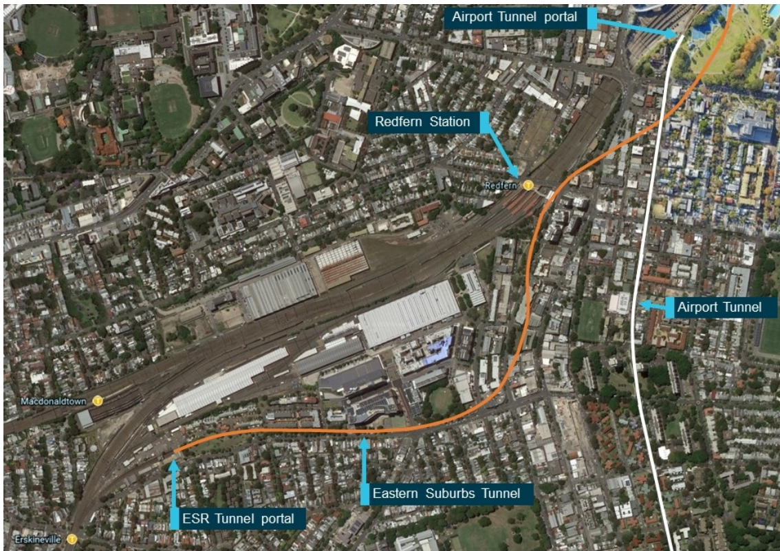
Figure 2: Eastern Suburbs Railway and Airport Line Tunnels
