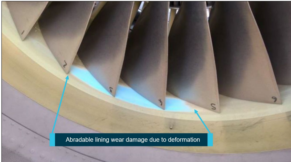
Figure 2: VH-YIW right engine abradable lining.
