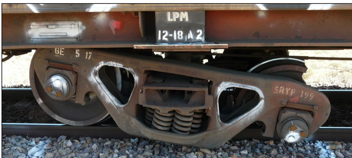
Figure 1: The ruptured and derailed wheel in situ
