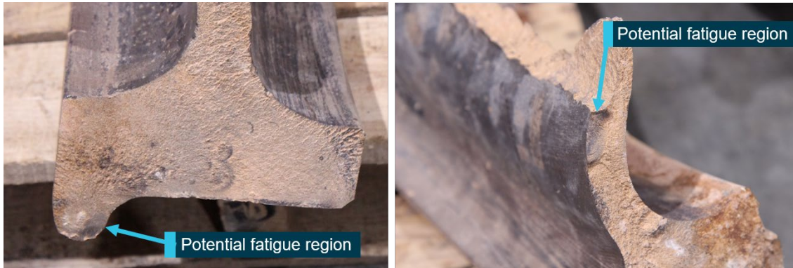
Figure 2: Two fatigue regions in the flange (left) and the plate (right)
