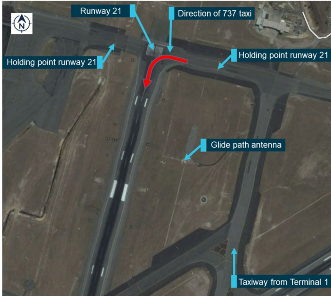
Figure 3: Perth Airport runway 21 showing location of glide path antenna, holding points and path of taxiing aircraft prior to take-off.
