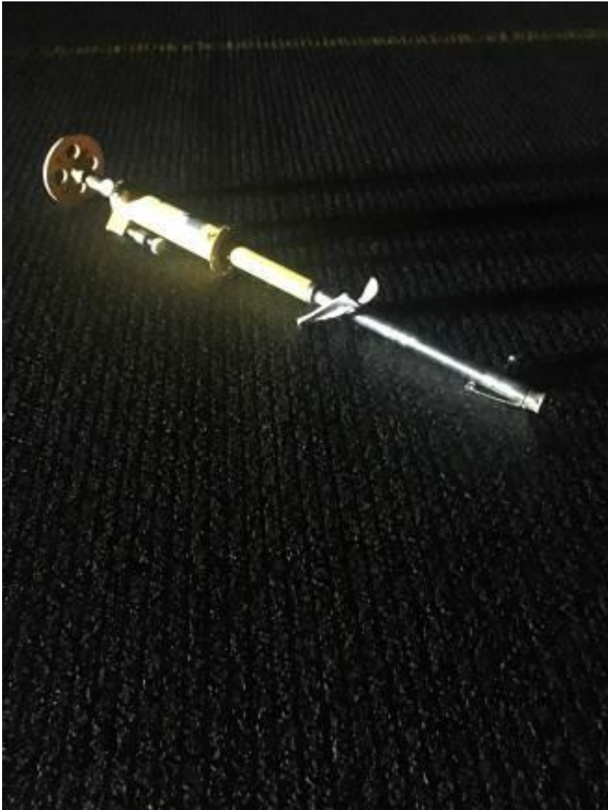
Figure 2: Tail strut as found on Sydney runway 16R post NJZ departure
