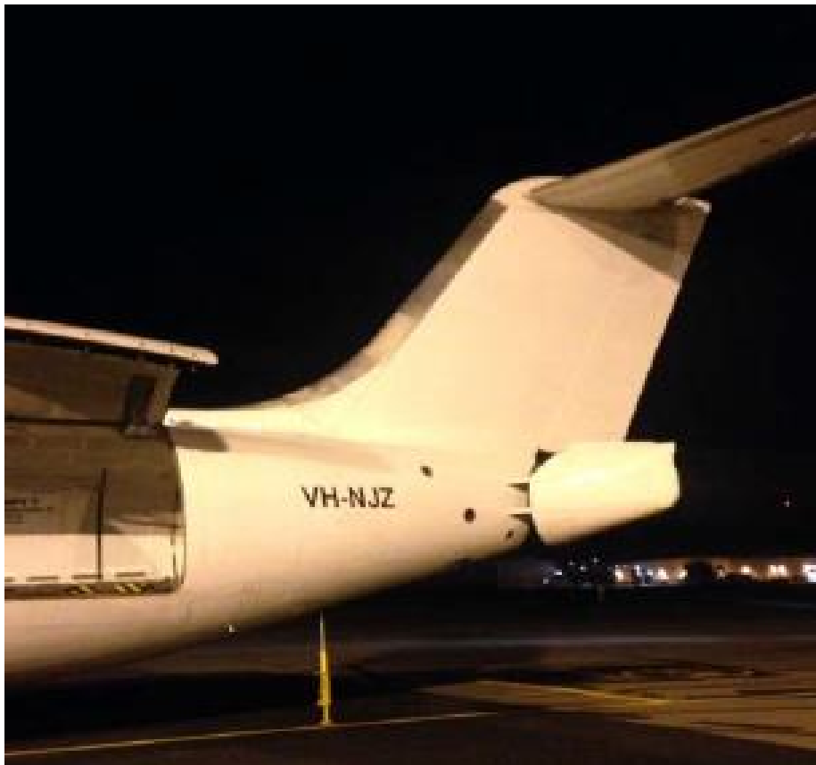
Figure 1: Example of a tail strut fitted to NJZ and showing opened freight door
